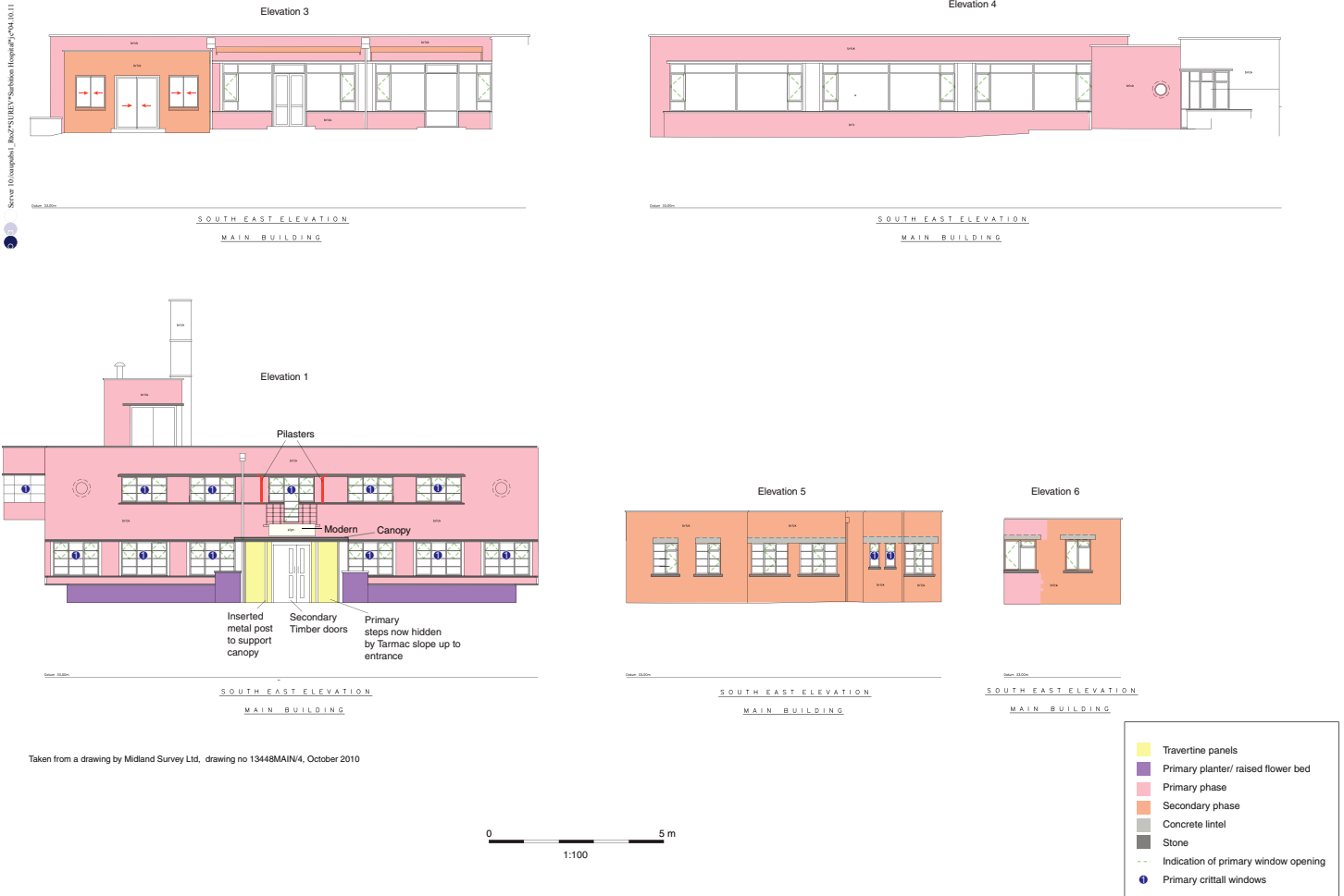
Figure 7: Elevations of main hospital: south-east
