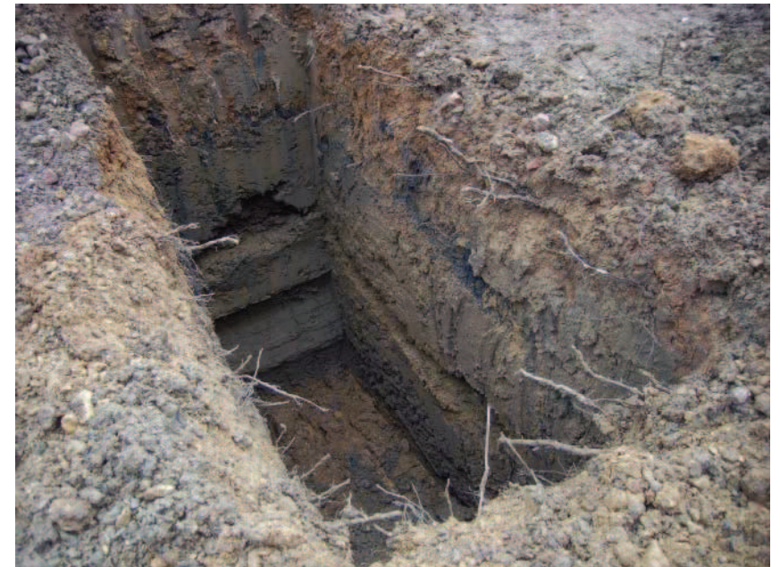
Plate : Maximum depth of gravel (4.6m) in Pad 30B
