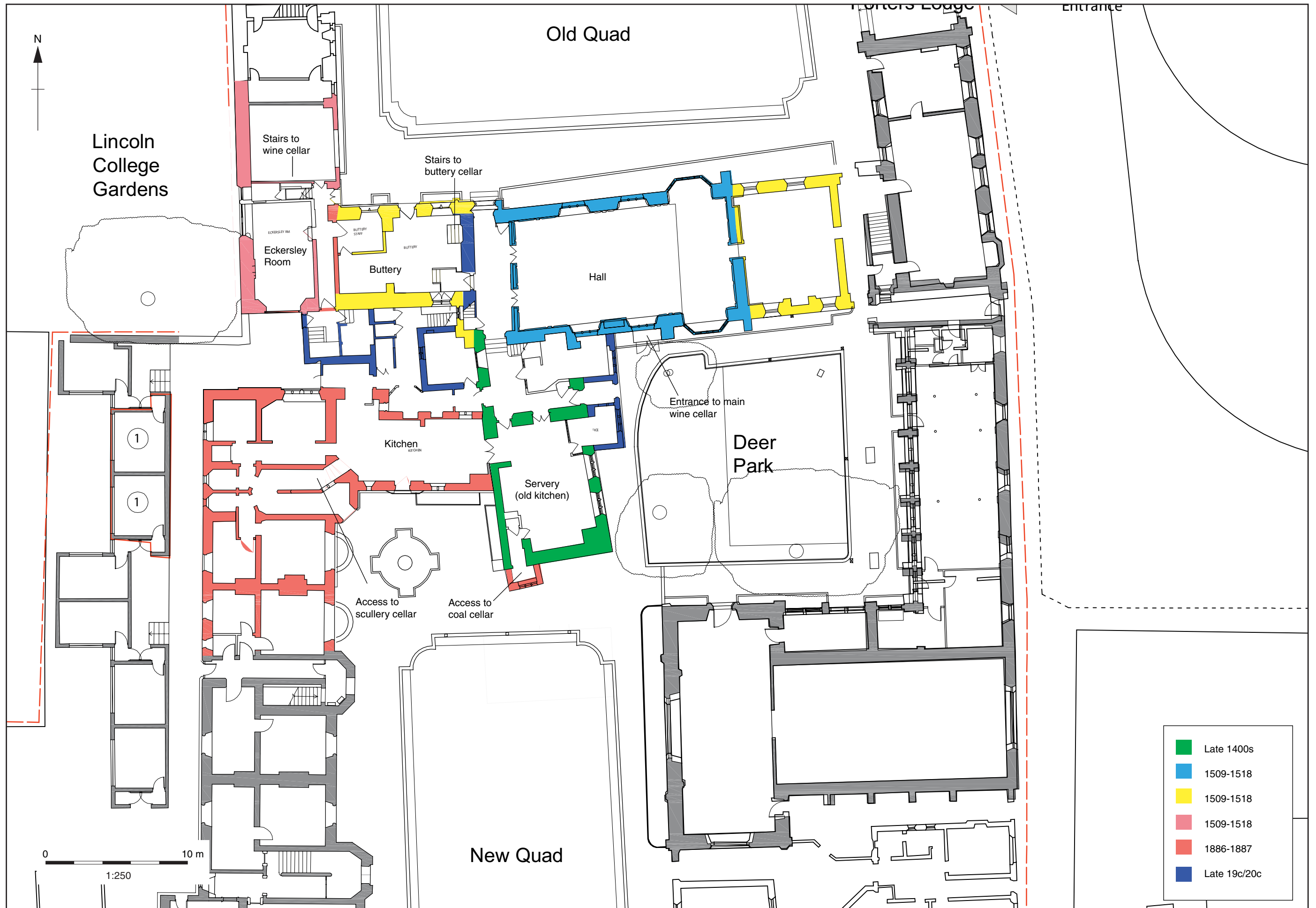
Figure 8: Plan of kitchen area showing extensions demolished as part of works and location of key features
