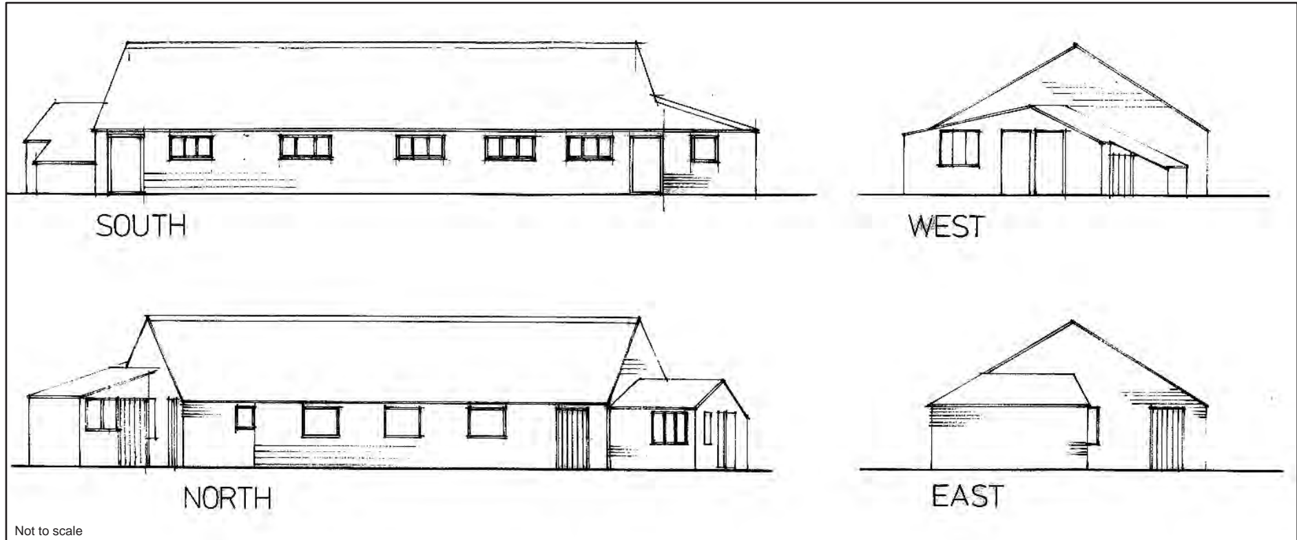
Figure 4: Elevations of the barn, based on drawings by Blenheim Design and Management
