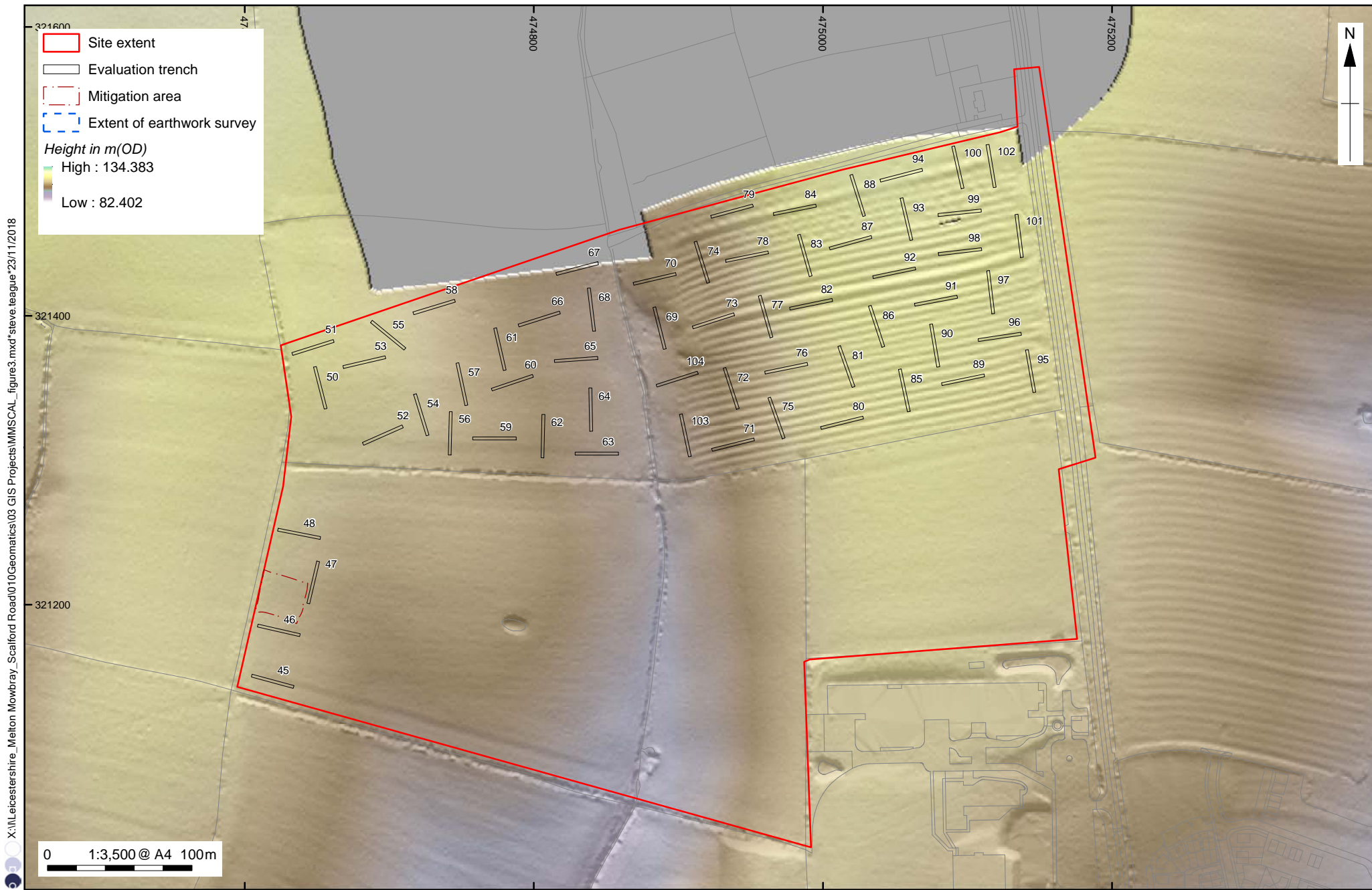
Figure 3: Result of LiDAR survey and earthwork survey, with multi-direction hillshade (D16)
