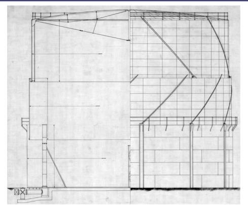
Appendix Figure 1: A section and elevation of an above-ground two-lift spiral guided gasholder
