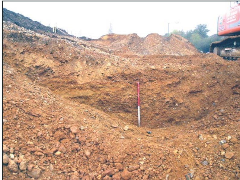
Plate 2. Fluvially bedded sand bed in situ within main gravel body [scale 1 m]
