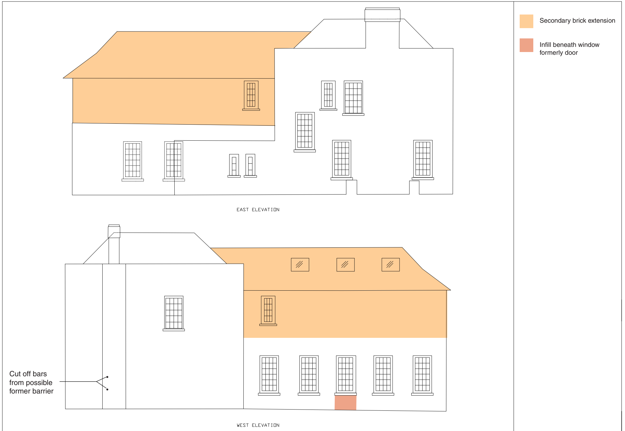
Figure 7: Elevations 2 (taken from a survey by Sterling Surveys and included in planning application document)
