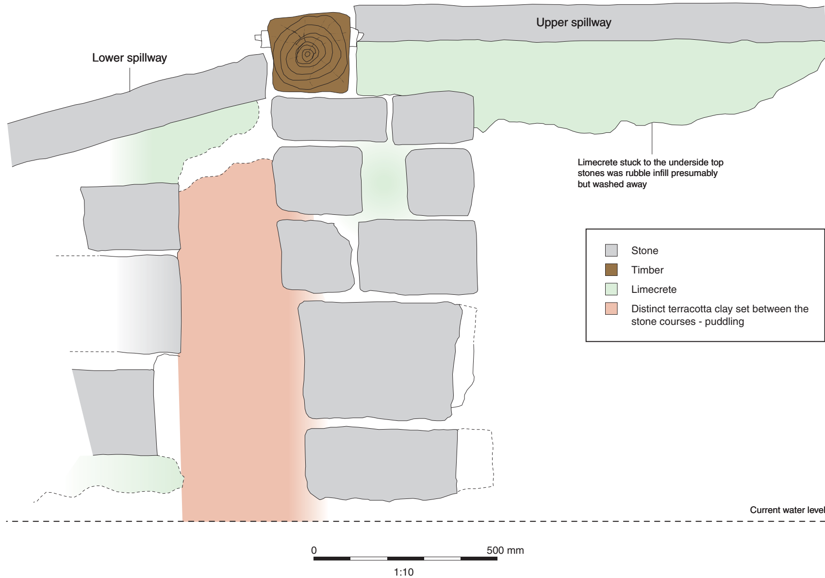
Figure 11: Section detail through spillway on east side of the island weir, looking south
