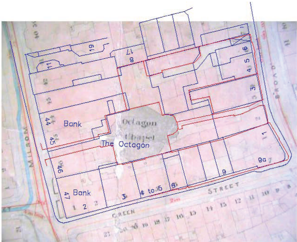
Figure 15. The 1886 property boundaries of 2 and 3, Broad Street in 1886 (in red line) superimposed on the 1853 Cotterell Survey, showing the alterations between those years, mainly the rationalisation of the vaults passage. This suggests that the southern boundary of no. 3 must have been rebuilt. While comparison with the 1901 lease plan suggests that the 1886 mapping is not quite accurate here they both show a realignment of the southern boundary of no 3, Broad Street. It was rebuilt on this new line in 1921. Curiously the modern OS, inaccurately, has reverted to Cotterell's line (blue lines).
