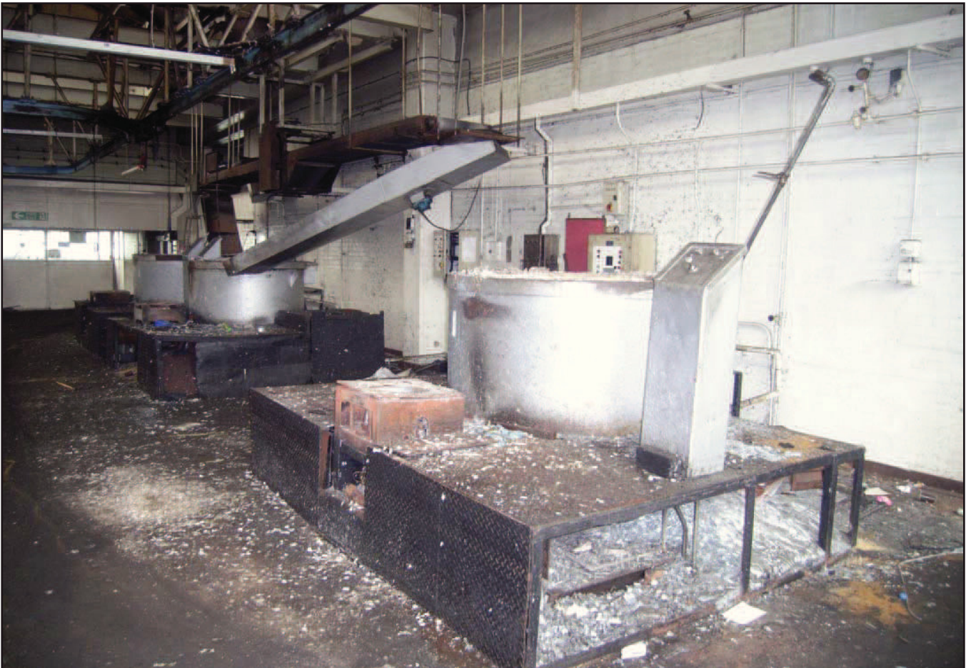
Plate 24: Zinc pots in foundry (1st floor Block C)
