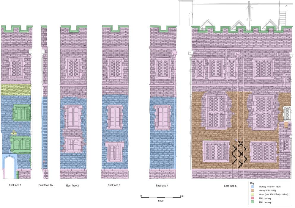
Figure 3: Hampton Court Palace, Chapel Court, East facing elevation (face nos 1-5) - Phasing of stonework and brickwork
