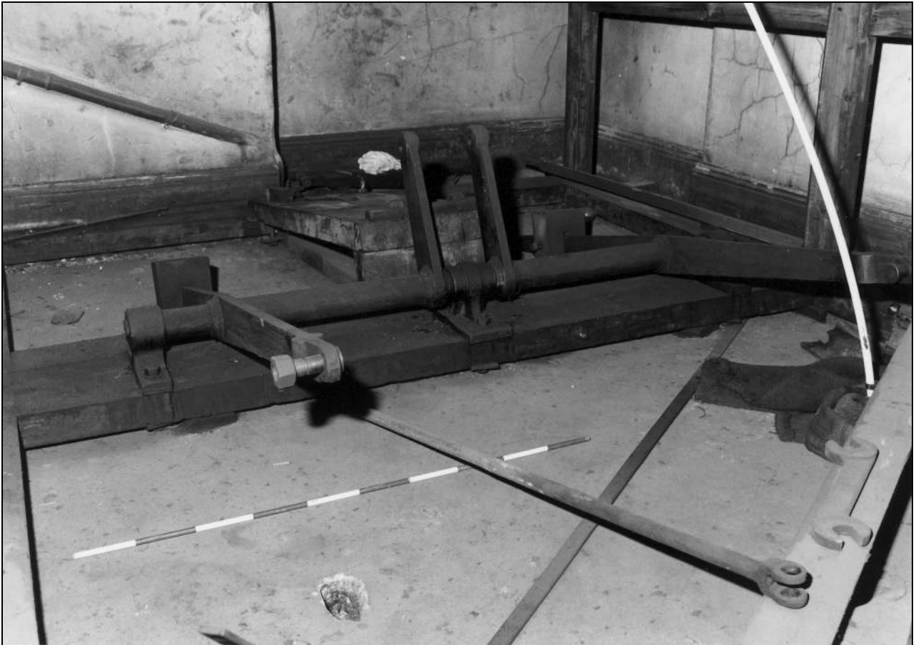
Photo 62: Cranks etc below organ bellows, from the west (film 7, frame 3)
