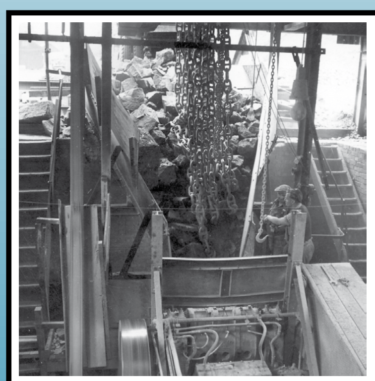
◀ In this photograph large stones are being poured into the crushing machine.
