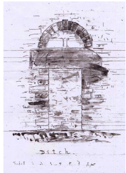
Plate 6 Drawing of the postern doorway in the south curtain wall by Willson
