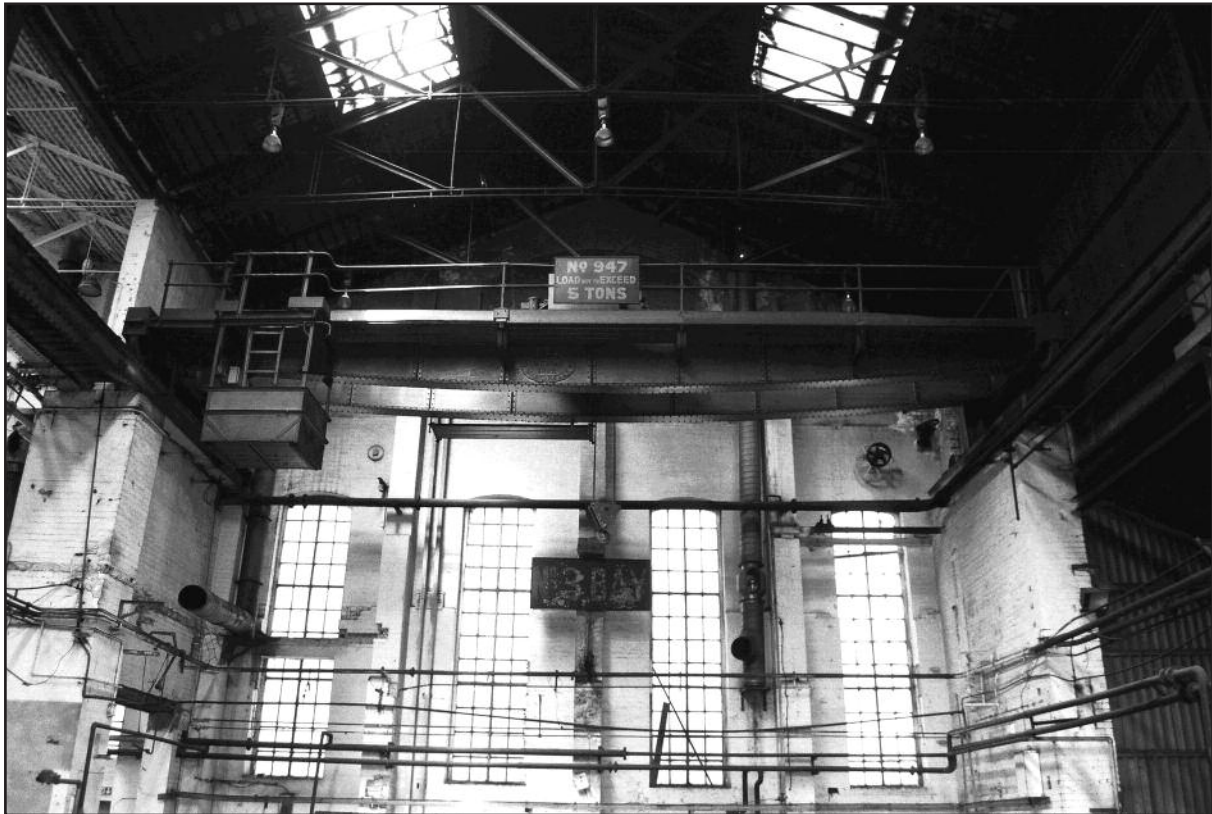
The early travelling crane from Park Iron Works, to a design of 1892 © ARCUS
