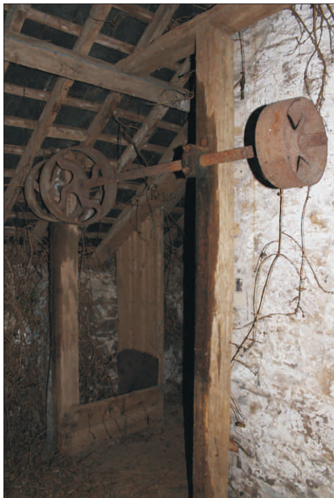
Plate 22: First-floor hayloft/engine house, detail of lineshaft and wheels, view from below, looking southeast
