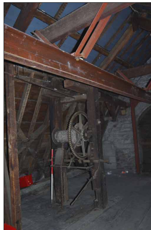
Plate 18: Cogs and chains of winch arm in the third-floor north store, looking northwest (1m scale)
