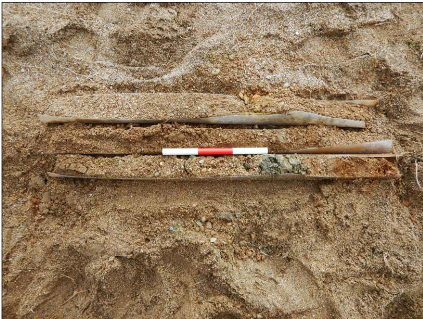
Plate 2: Showing borehole sleeves with recovered sand layer sequence (scale 1m)
