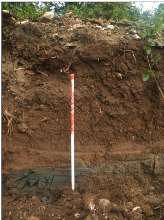
Plate 3: Representative section of riverbank alluvial deposits beneath topsoil. View to northeast (scale 1m)
