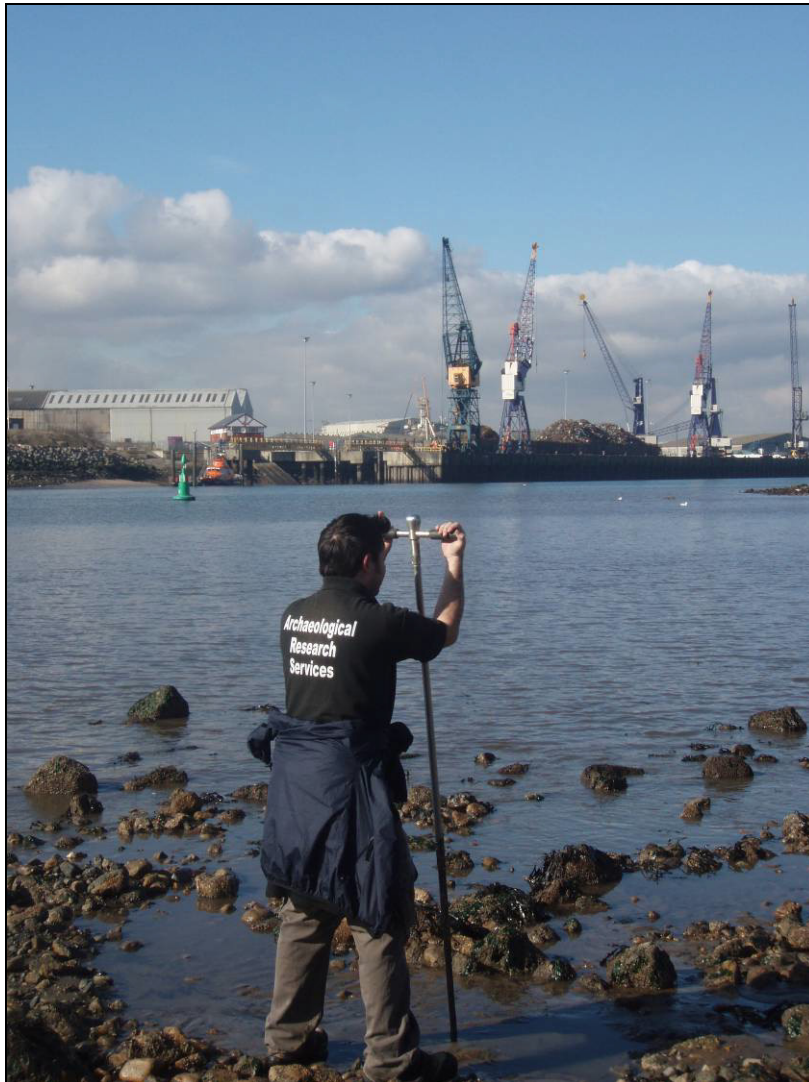
Fig 4.4 Undertaking sediment coring at Hartlepool Bay, Teeside.
