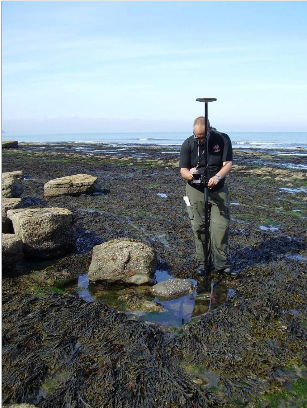
Fig 3.6 Recording of a rock cut feature with the Magellan GPS equipment, possibly a fish trap or “hulley”, on the foreshore at Hummersea, North Yorkshire (see Chapter 5).
