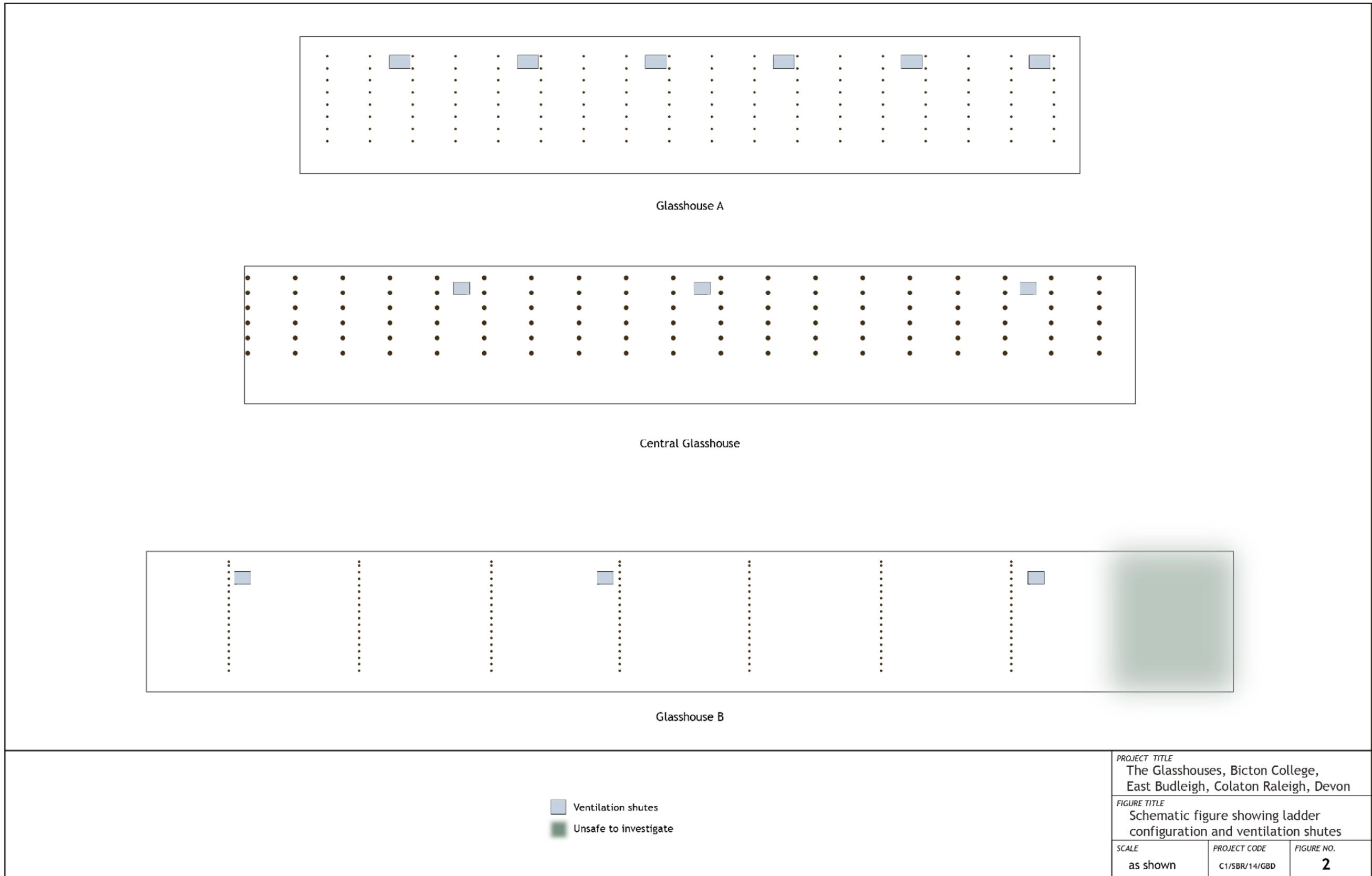
Figure 2. Schematic figure showing ladder configuration & ventilation shutes
