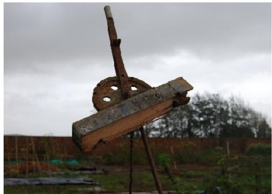
Plate 8. Gear of roof opening mechanism fixed to wooden bracket, with long pole to connect to roof & pin with chain to lock the gear
