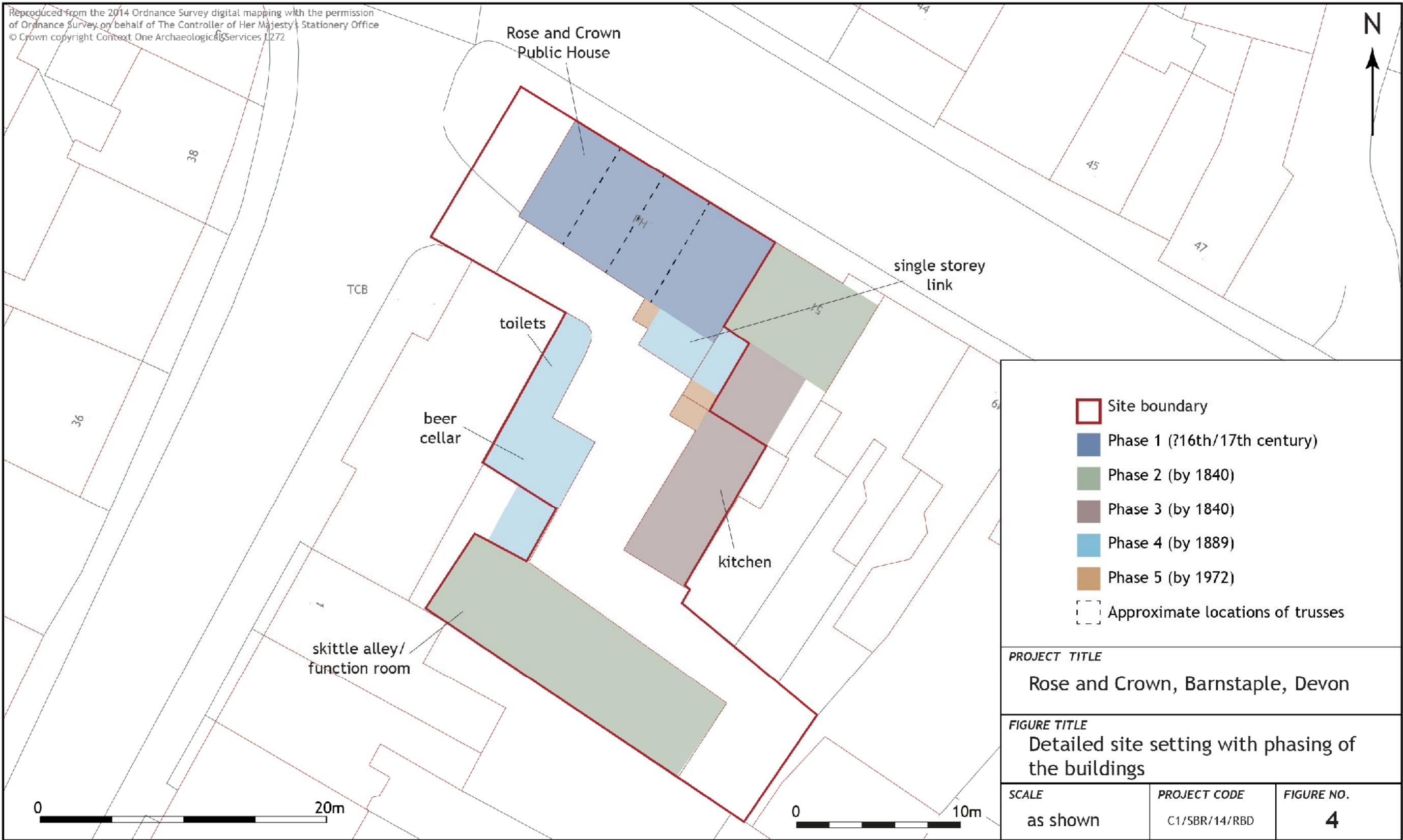
Figure 4. Detailed site setting showing phasing of building
