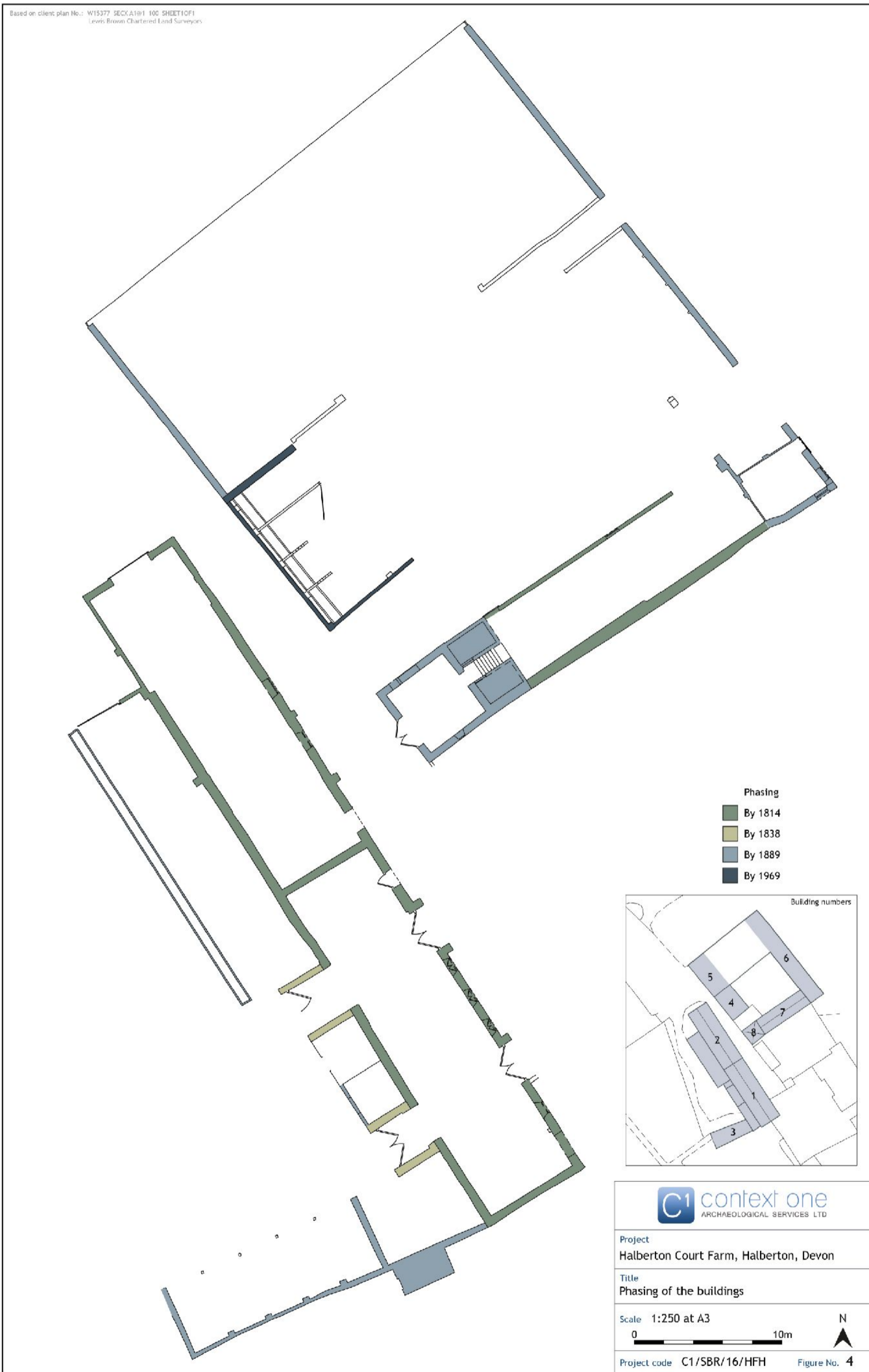
Figure 4. Phasing of the buildings
