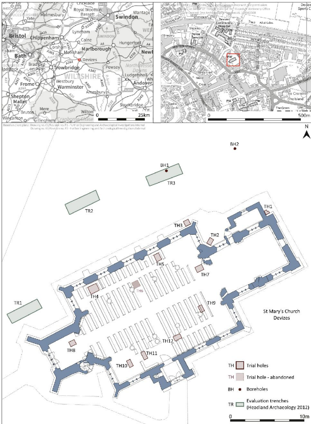
Figure 1. Site setting with trial hole and borehole locations
