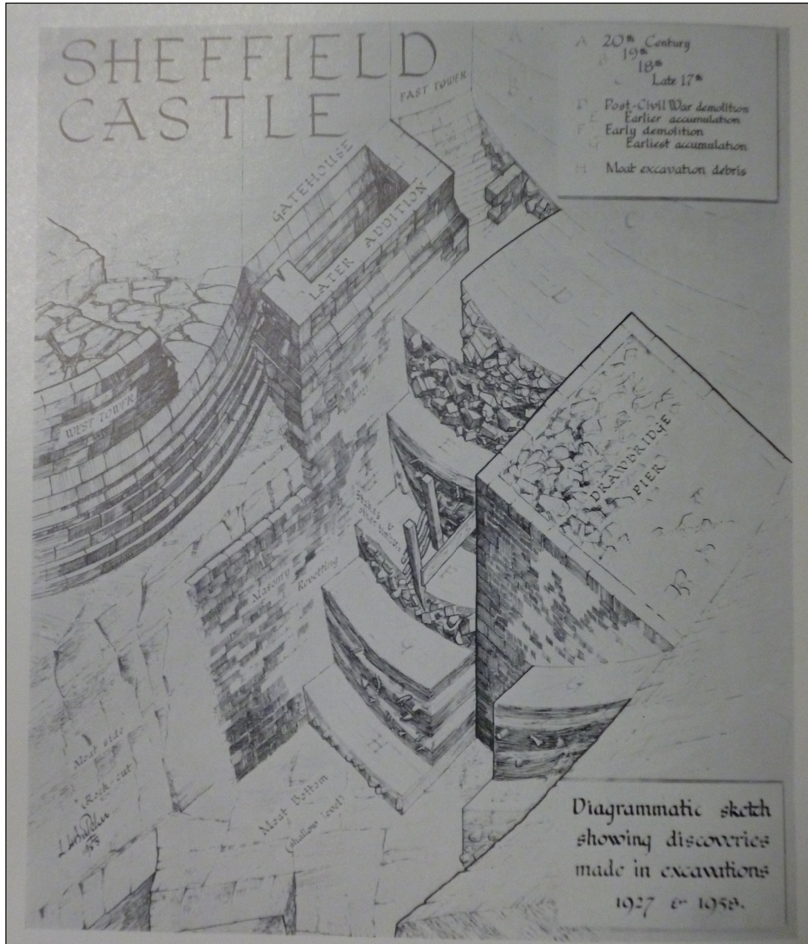
Isometric reconstruction of gate structures. Source: Sheffield City Museum 1960 City of Sheffield: The City Museum Annual Reports 1958-60 , 9 & 12.
