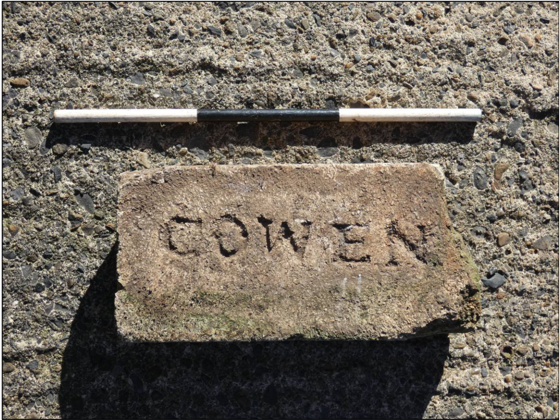
Plate 11: Hand-moulded firebrick, stamped COWEN, recovered during excavations (photo 5/236).
