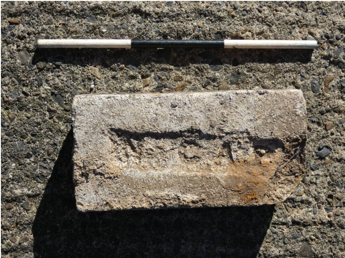
Plate 12: Hand-moulded firebrick, stamped N CAP, recovered during excavations (photo 5/237).
