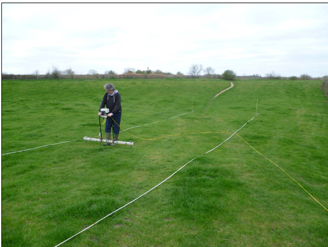
Plate 2: Resistance survey in progress, March 2019.
