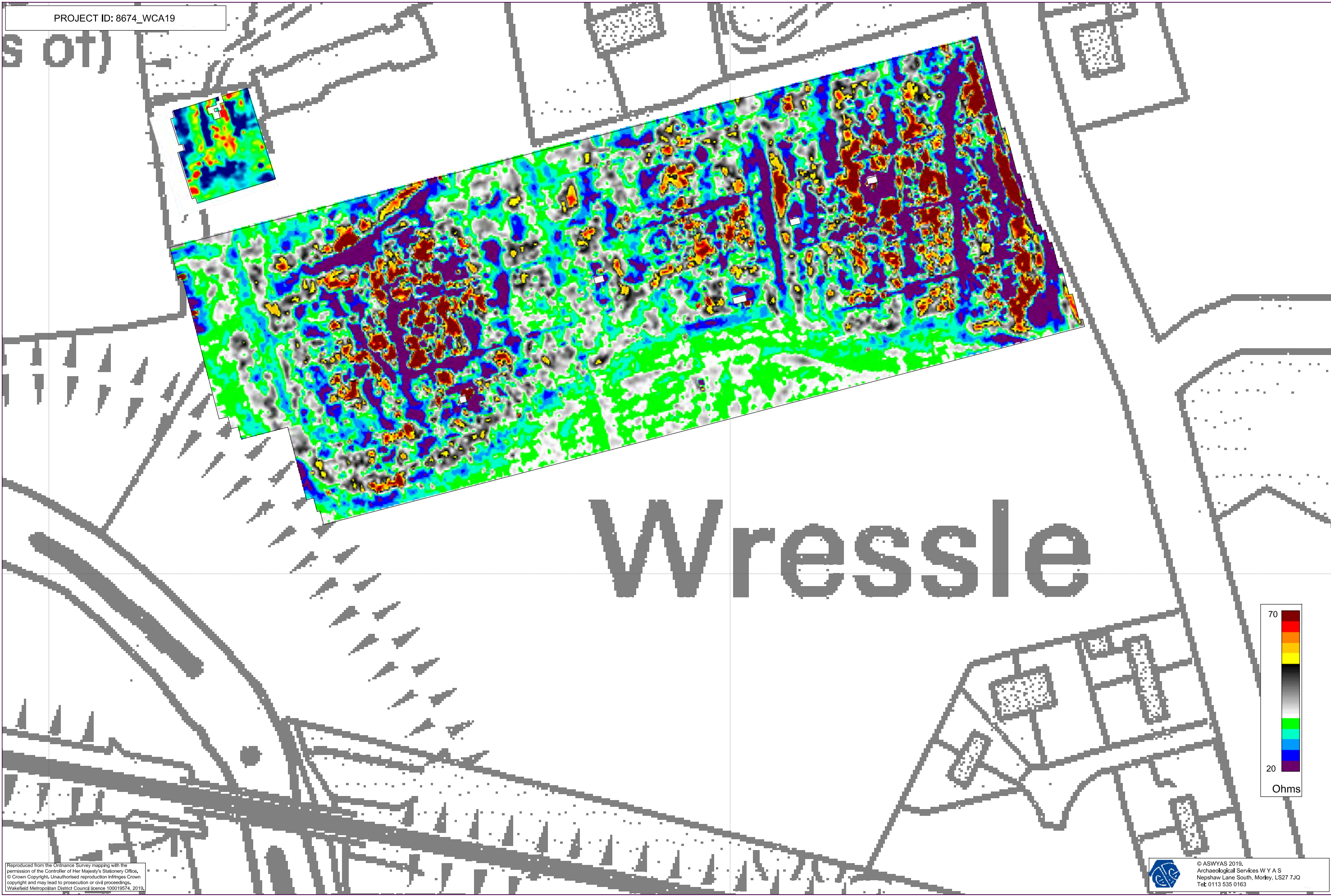
Fig. 8. Processed earth resistance data (1:1000 @ A3)
