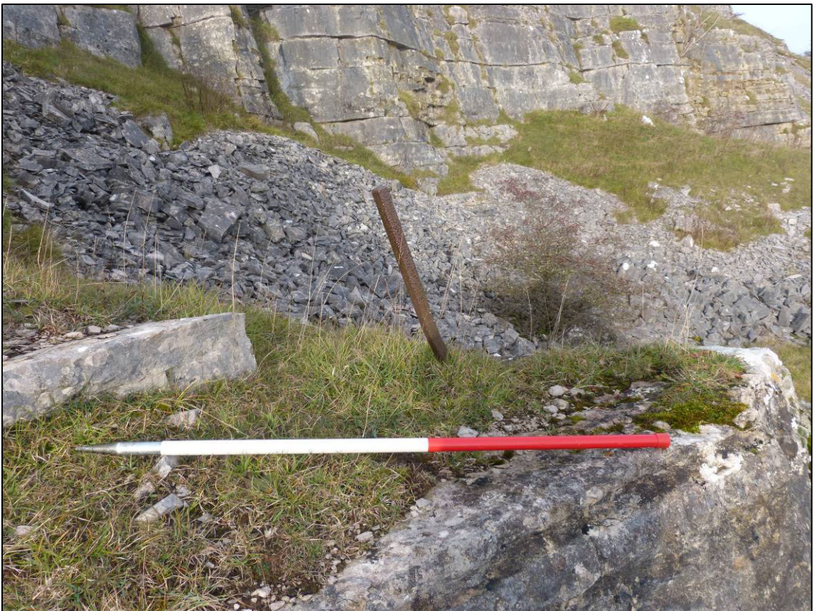
Plate 23: Smardale quarry, jumper in main quarry face (Site 105), looking N (photo 2/141).
