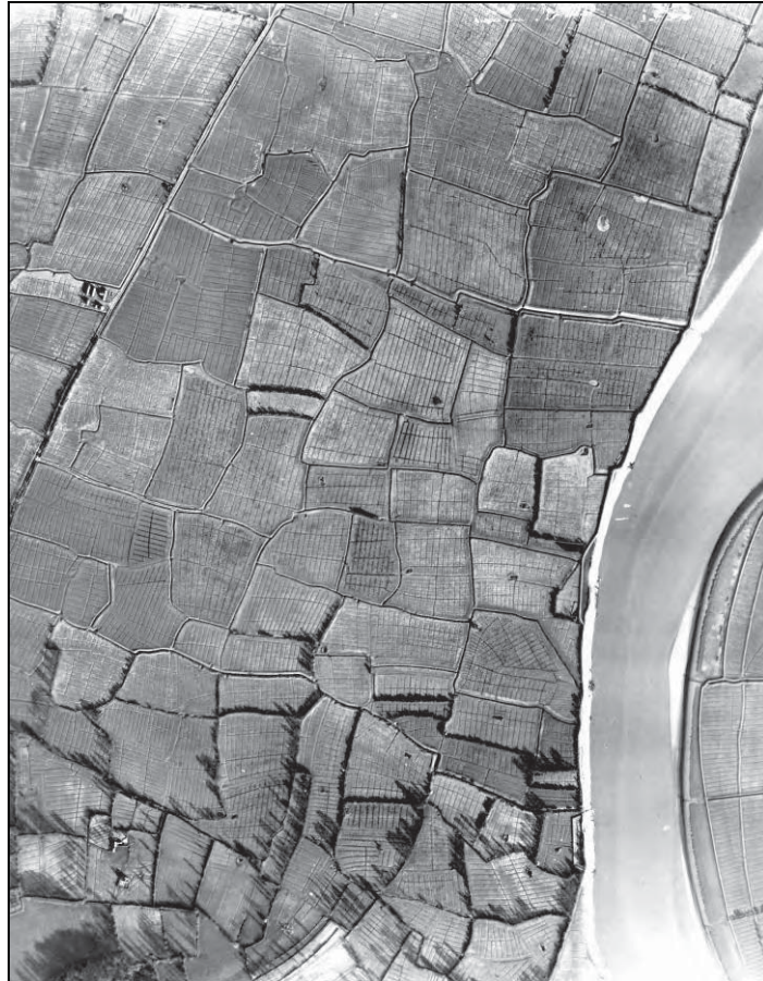
Figure 2.10. The irregular fields which cover much of the Somerset Levels. The fields are separated by larger ditches and rhyes and the fields show the network of cut ditches known as grips, which are part of medieval and/or post-medieval land improvement.
