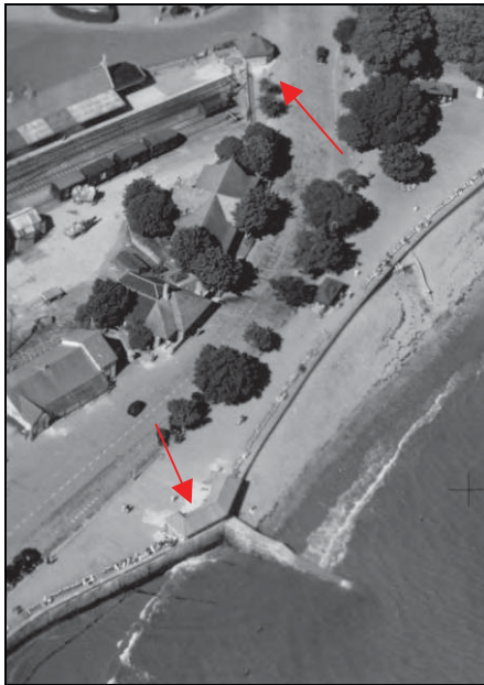
Figure 10.6. Second World War military structures on Minehead promenade. Centre of the photograph is a concrete infantry section post. Top centre is a pillbox disguised as a kiosk outside the railway station.
