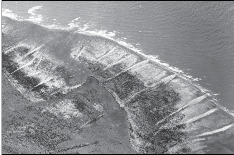
Figure 5.23. Linear pebble-built structures on Madbrain Sands, Minehead that may limit longshore drift.
