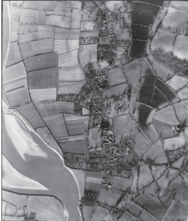
Figure 9.34 Flooded areas to the east of Longney ('long island') indicate a possible former channel of the River Severn. The drained fields are protected by three linear earthwork banks. To the west of the village, a series of sea banks record successive land reclamations.
