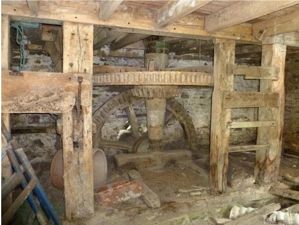
South mill hurst and primary machinery, with bridge post and tentering adjuster on left
