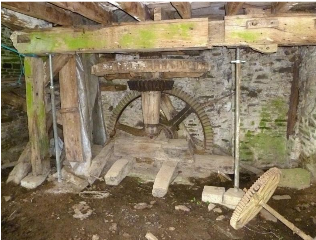
North mill: remains of hurst and primary machinery
