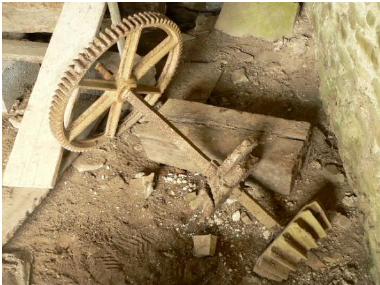
Displaced drive shaft (1). The iron bevel gear meshed with the pitwheel and the spur gear with the pinion on drive shaft (2)
