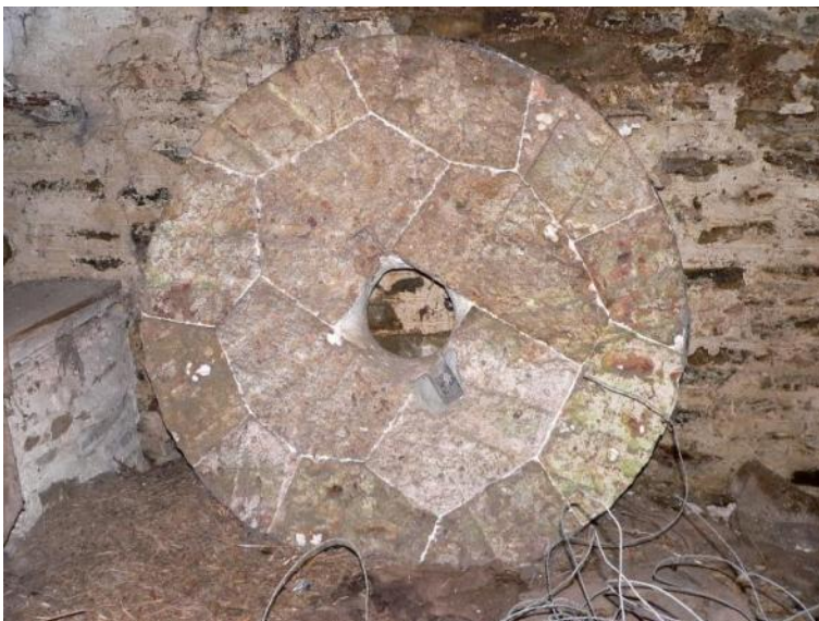
Displaced French burr millstone in south mill
