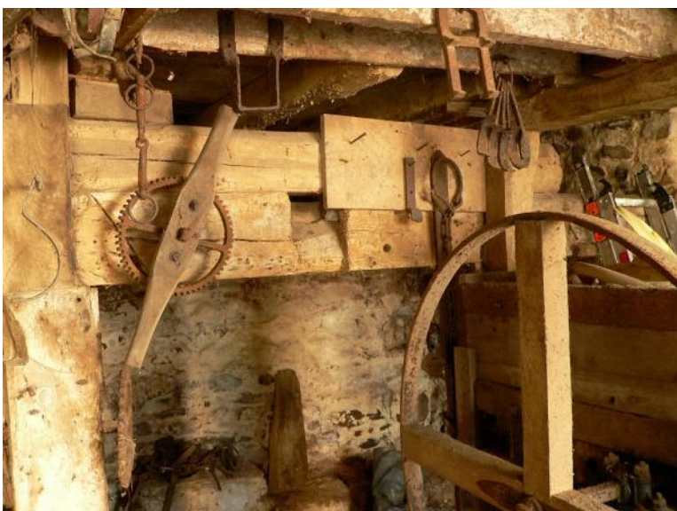
Hurst, bridging and tentering gear to upstream millstones
