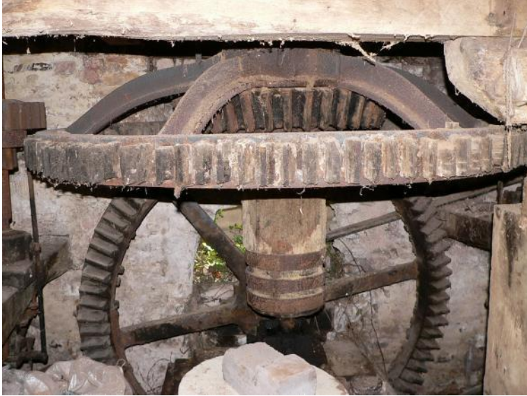
Primary gearing, showing dished arms of spurwheel
