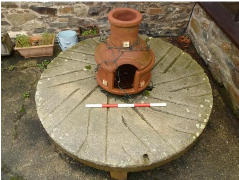
Peak runner stone outside mill house (half metre scale)
