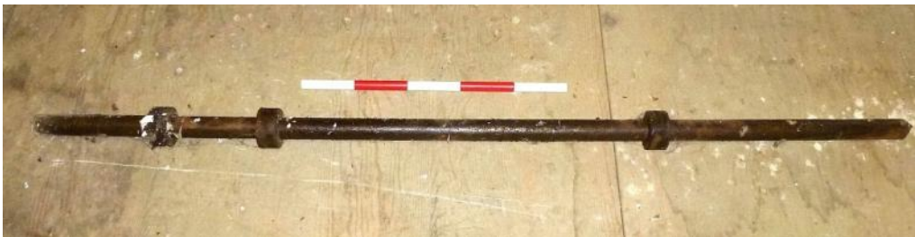
Drive spindle from grain cleaner or flour dresser (half metre scale)
