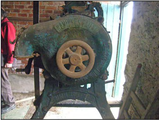
Crushing and rolling mill standing by the northern door of the interior South Range, first section (from E-W), with a maker's plate identifying its manufacturer, Henry Bamford and Sons, Uttoxeter.
