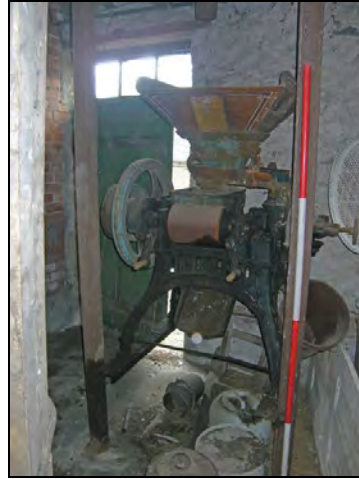
Crushing and rolling mill standing by the northern door of the interior South Range, first section (from E-W), with a maker's plate identifying its manufacturer, Henry Bamford and Sons, Uttoxeter.
