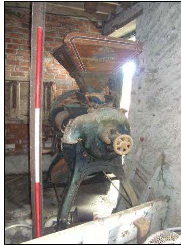
Crushing and rolling mill standing by the northern door of the interior South Range, first section (from E-W), with a maker's plate identifying its manufacturer, Henry Bamford and Sons, Uttoxeter.
