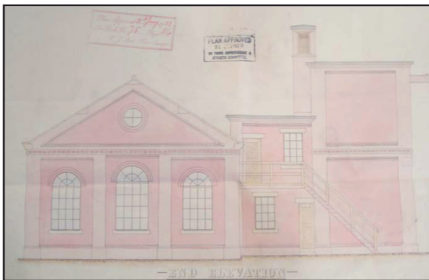
Illus. 23: Building plan showing the end elevation of the new electric pumping house as proposed in January 1923 for Newcastle and Gateshead Water Company (TWM T186/2070).
