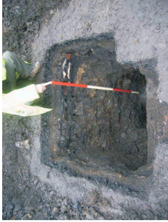
Illus. 32: Test pit within the area of the proposed new development, showing disturbed ground to over 2m depth.
