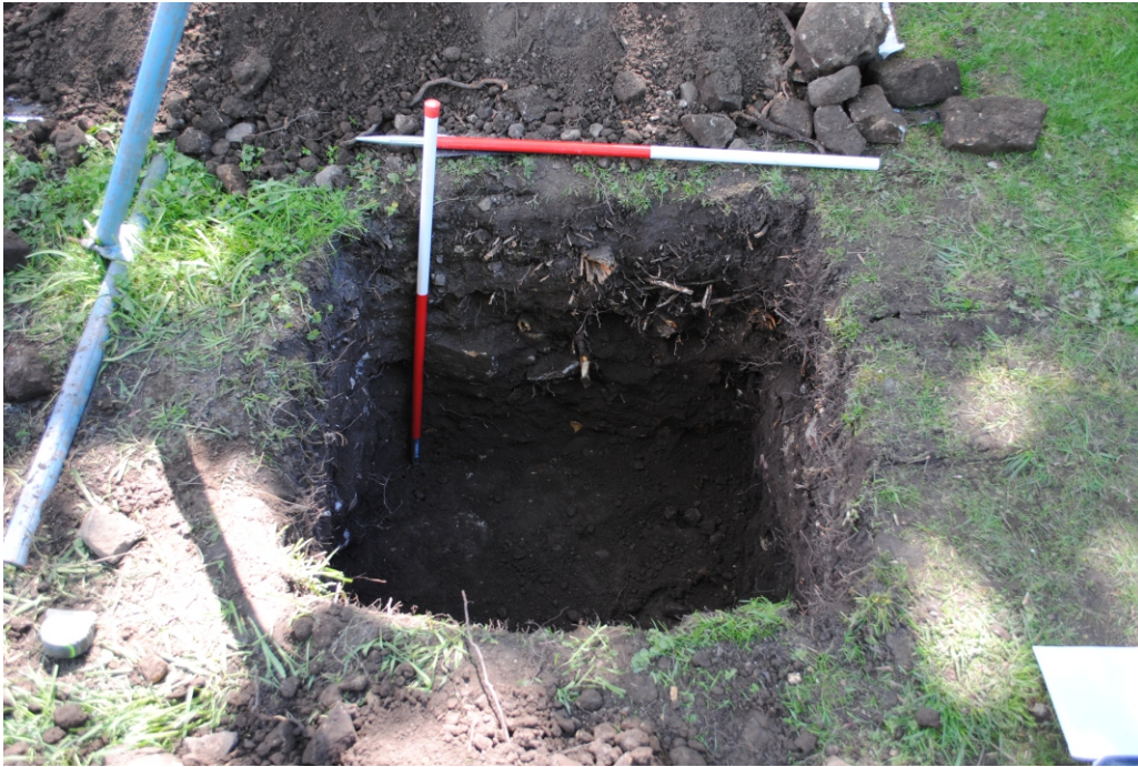
Photo 01. Soakaway pit 1 looking south.
