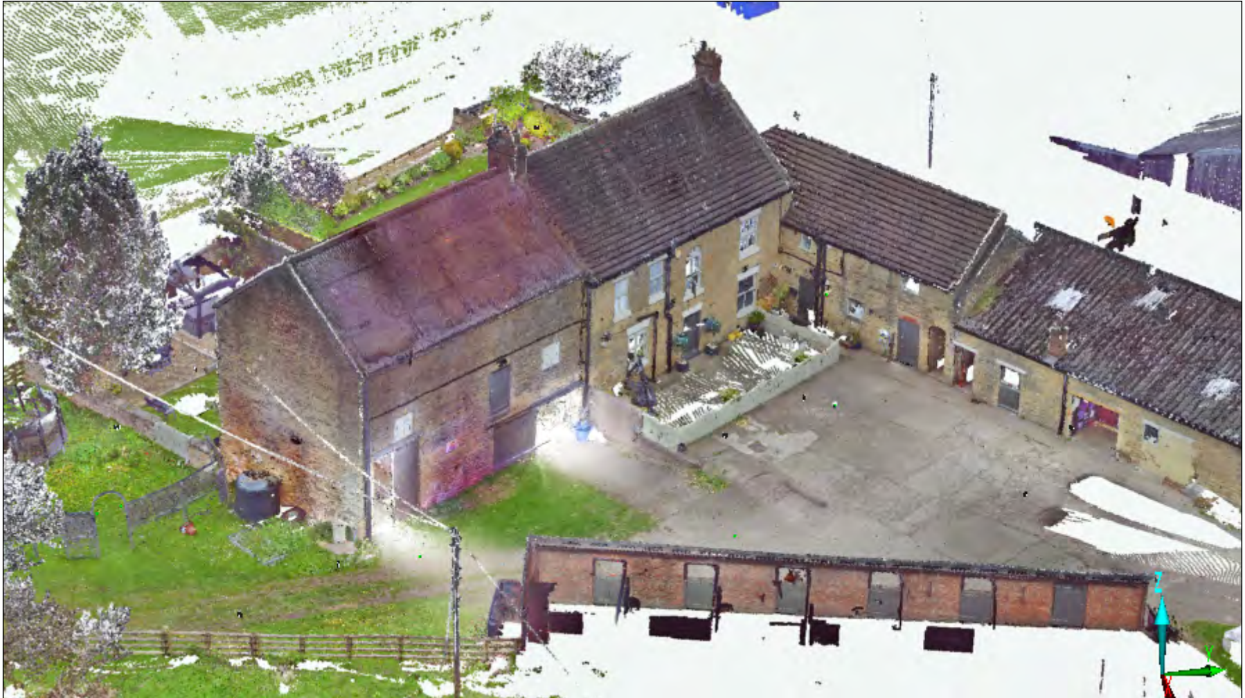
Illus. 19: Digital 3D scan of Ricknall Mill Farm, looking west. Produced by Gianluca Foschi in April 2022.
