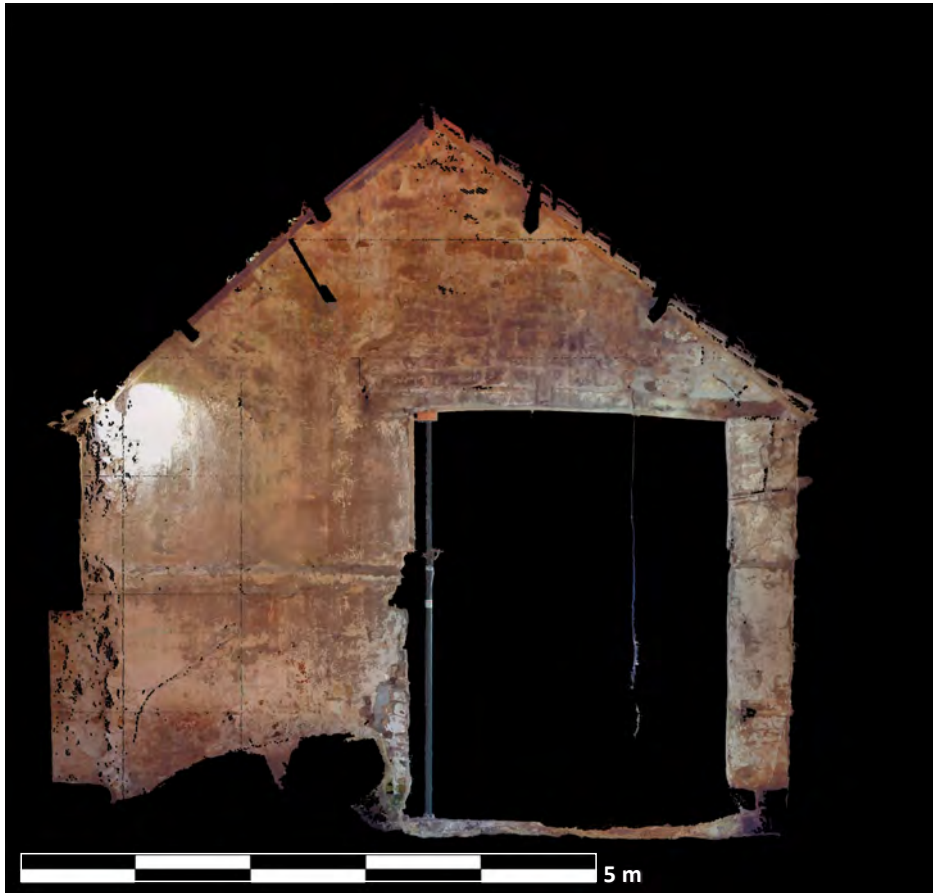
Illus. 19: Digital Scan of the east elevation of the Medieval Chapel, forming the intersection with the Central Barn in the North Range, Walworth North Farm, by Gianluca Foschi, April 2022.
