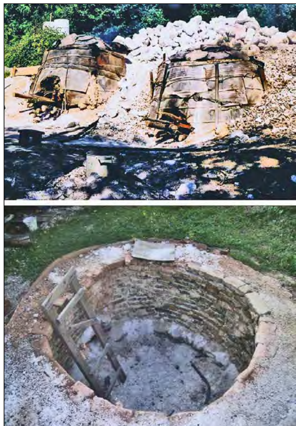
Illus. 05_06 a&b: Traditional European flare kilns. Although superseded in Northern & Western Europe, traditional flare kilns of the form once used in Northumberland are still used by small-scale producers in Southern and Eastern Europe, where they are used to produce pure forms of lime, often from superior forms of limestone, untainted by the by-products of burnt fuel. The pure lime products are often sold in small quantities directly to consumers, or in larger quantities to middlemen or professional builders, the majority of whom use it as lime wash. The upper photograph shows two kilns built into a road embankment with a supply of limestone dumped by the roadside. The kilns, of 1-2 tonnes capacity, are being fired with beachwood stoked through an opening into the firing chamber, over which the limestone blocks are stacked to form a temporary vaulted floor. The top of the kiln is loosely covered with tiles and metal sheeting during firing, which takes approximately a day and night of continuous stoking, towards the end of which flames shoot out of the top of the kiln. The lower photograph shows an empty kiln with brick lining and ledge from which the temporary limestone vault is sprung.
