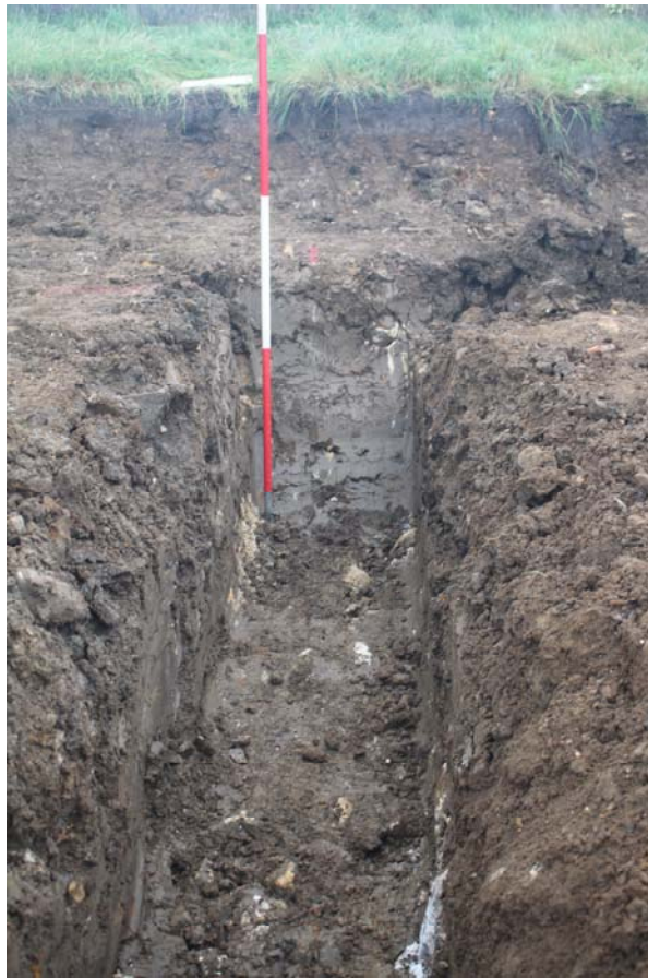
Plate 3: excavated trench from plot 1 showing the glacial till, looking north
