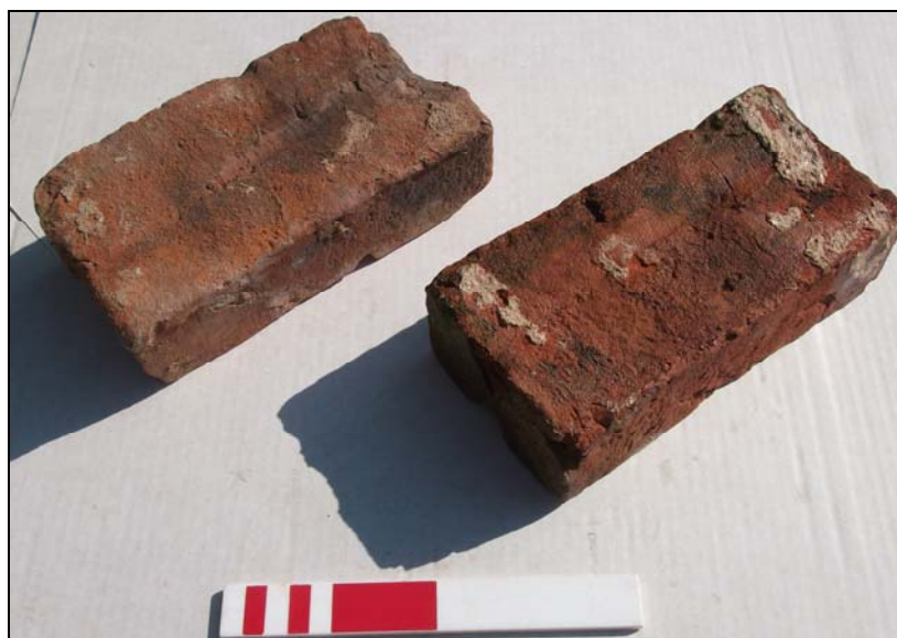
Plate 34, 66: Detail of the slope moulded bricks of the house (right) and the barn (left)
