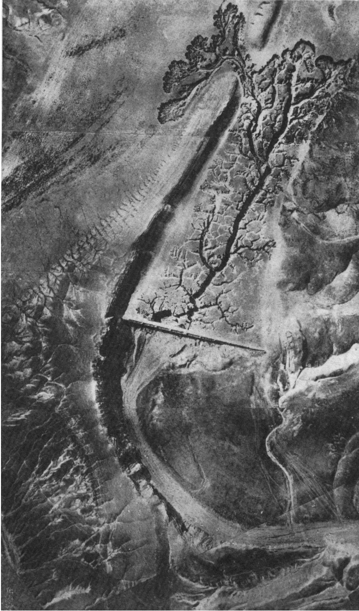
Fig. 4.13: Aerial photo of the Harbaqa dam, Syria, showing the extent of the silting of the reservoir in the 1930s [Poidebard 1934, plate 34].
