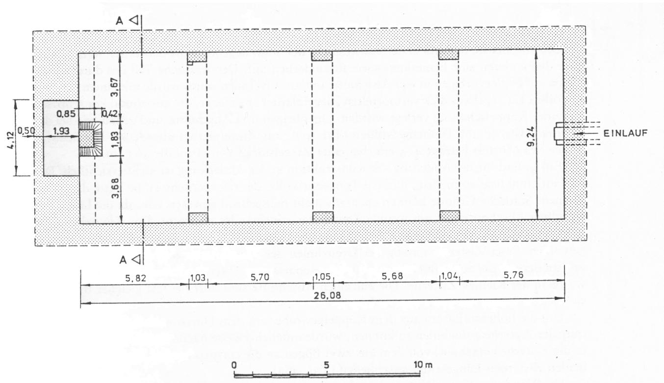
Fig. 7.28: Plan of the 'Small Reservoir-Cistern', Resafe [Brinker 1991, fig. 6].
