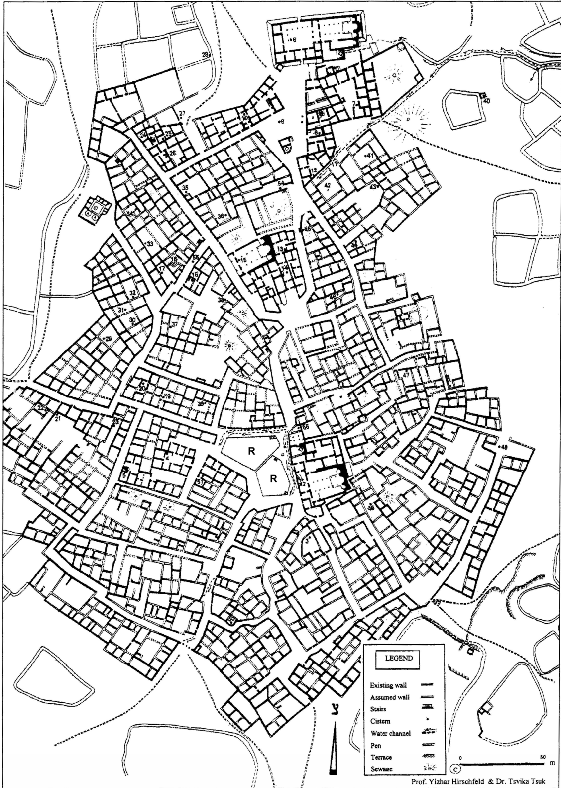
Fig. 7.36: Plan of Sbeiteh showing the locations of water management installations (R = reservoir) [Tsuk 2002c, map 1].
