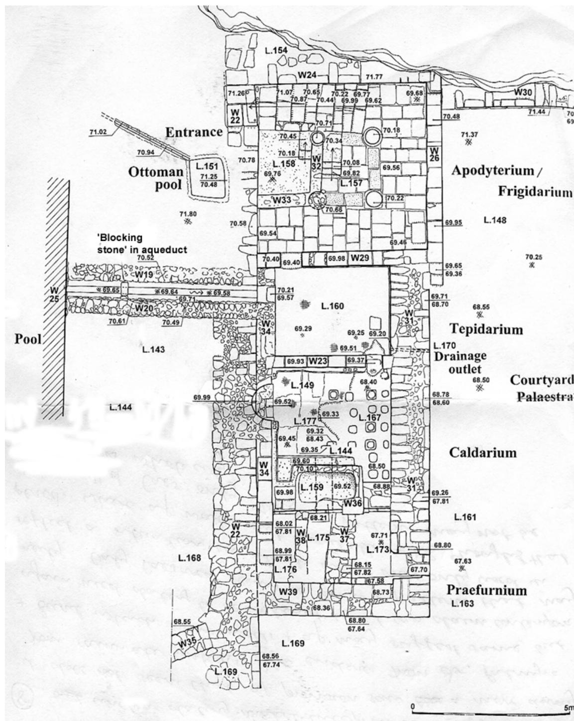
Fig. 8.13: Plan of the main bathhouse area, Ramat Hanadiv [after Hirschfeld 2000, fig. 180].
