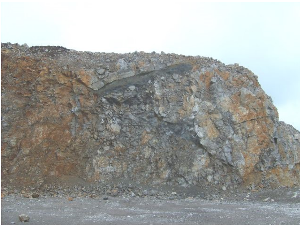
Plate 32 – View facing east of lift 'D', Old Moor Quarry. At centre are a number of sediment choked faults.
