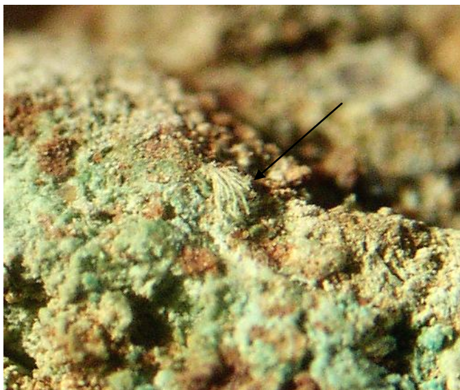
Non-mineralised fibre tuft among copper corrosion products (X16 image)
