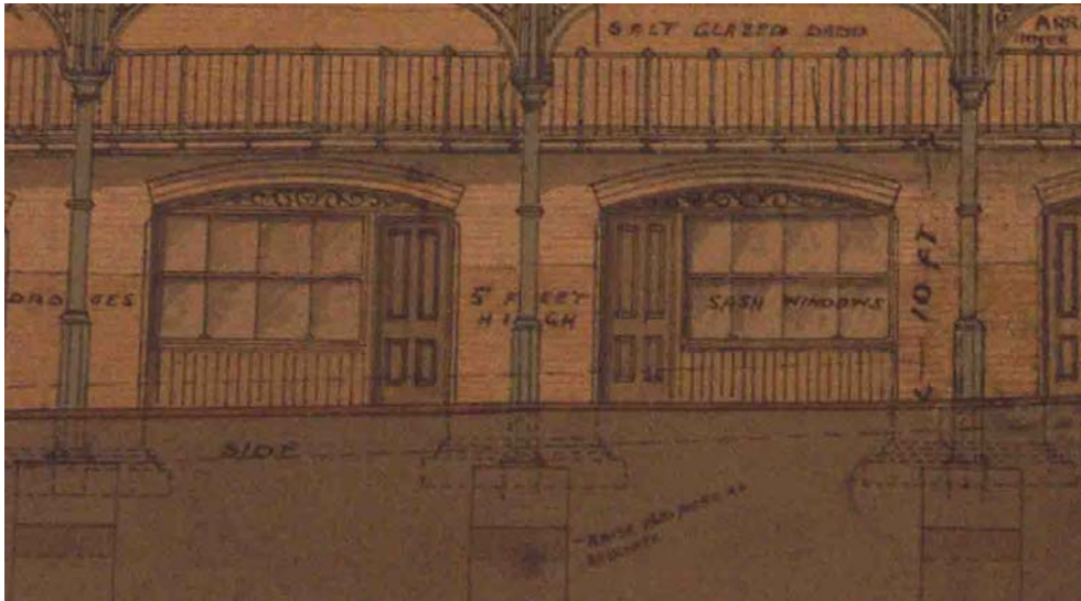
Plate 7: Showing original architects drawing of the second 1888 Market Hall design with instruction to “raise old peers as requested” relating to the brick pillars (my emphasis). Note also the blocks supporting cast iron roof support columns. (Courtesy of Rotherham Archives)
