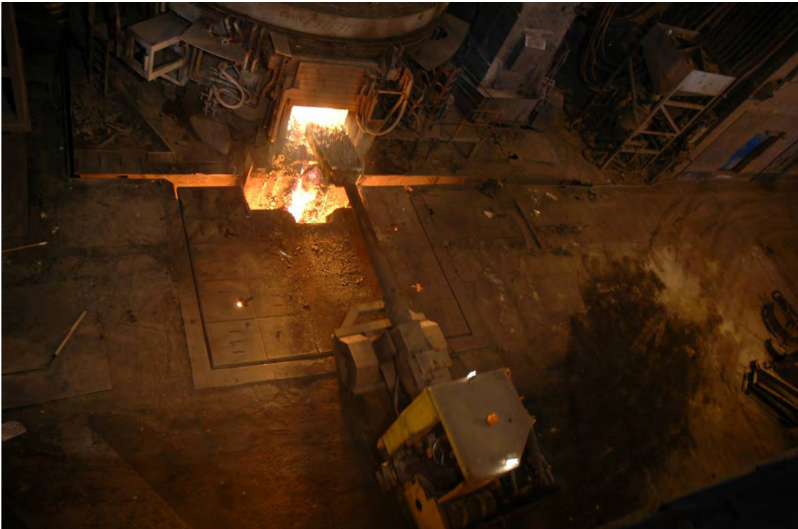
Plate 57: Alloys are charged into the furnace through the slagging door. These combine with the molten steel to produce stainless steel
