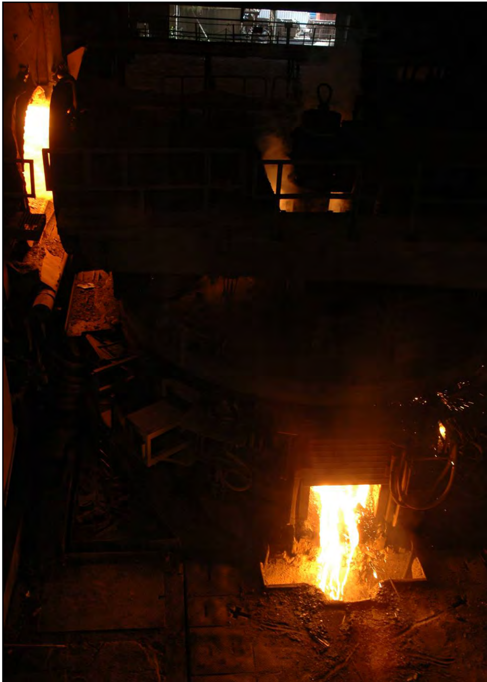
Plate 56: The furnace is tilted and the molten slag is poured into the ladle
