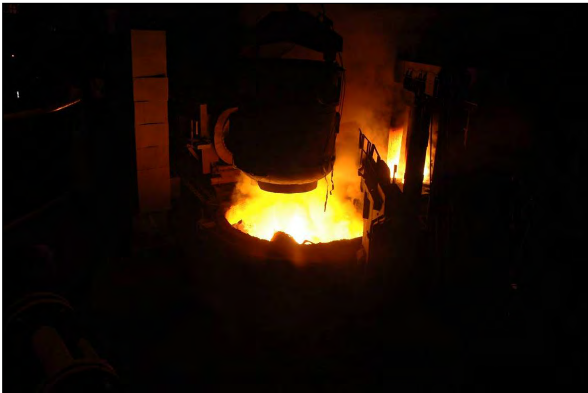
Plate 47: The scrap is charged into the furnace
