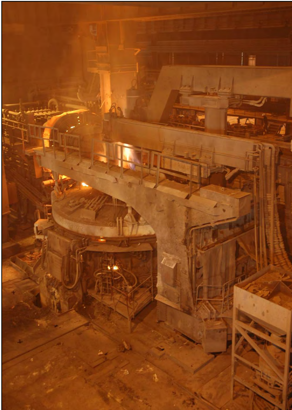
Plate 44: The arc stabilizes as the scrap begins to melt and the process continues
