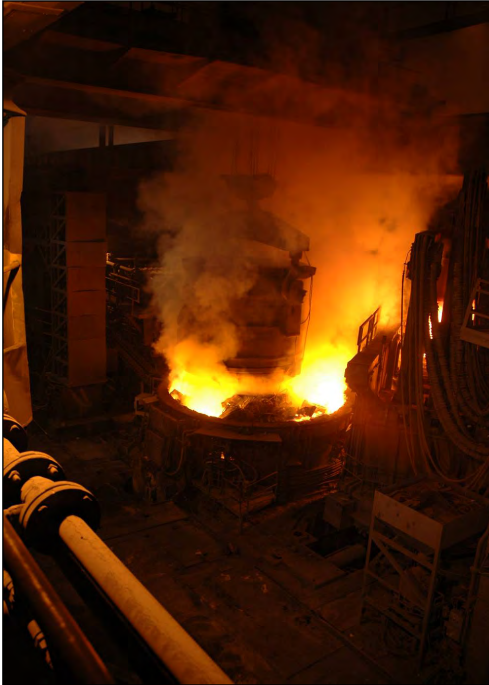
Plate 41: The scrap is tamped into the furnace in order to allow the furnace roof to re-close
