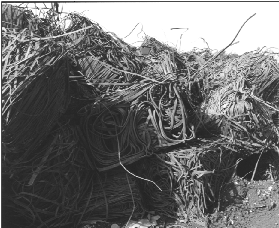
Plate 20: Detail of baled basic steel shred (13:6)
