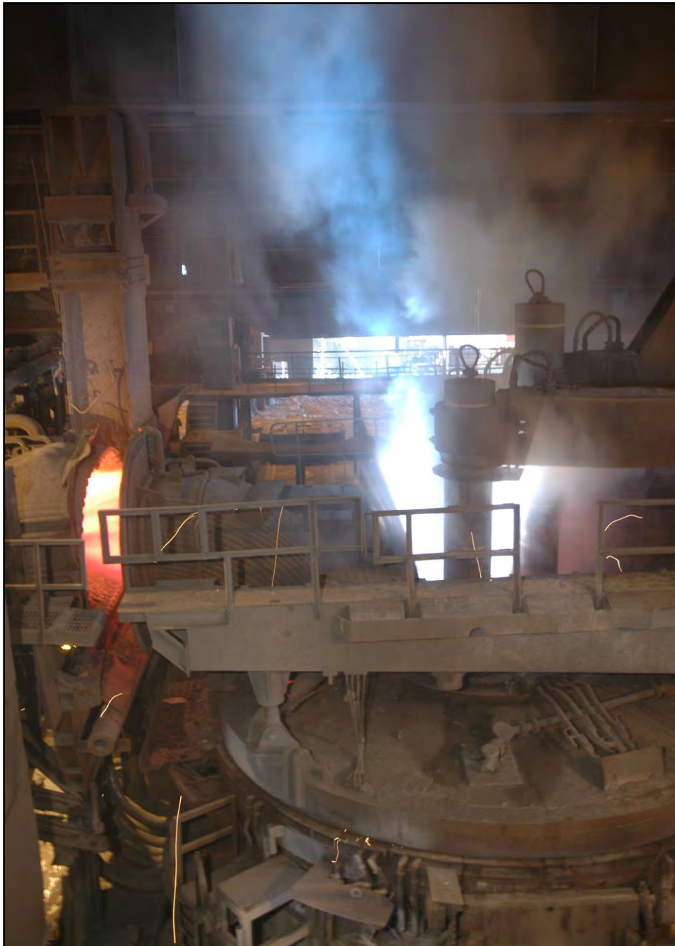
Plate 43: The electrodes are lowered and the arc is struck into the scrap, starting the melt
