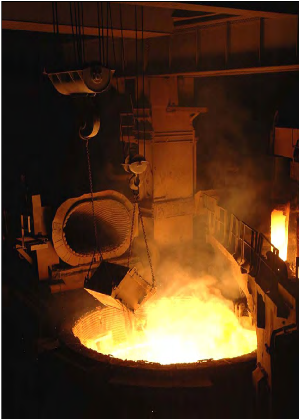
Plate 52: The limestone is tipped into the melt
