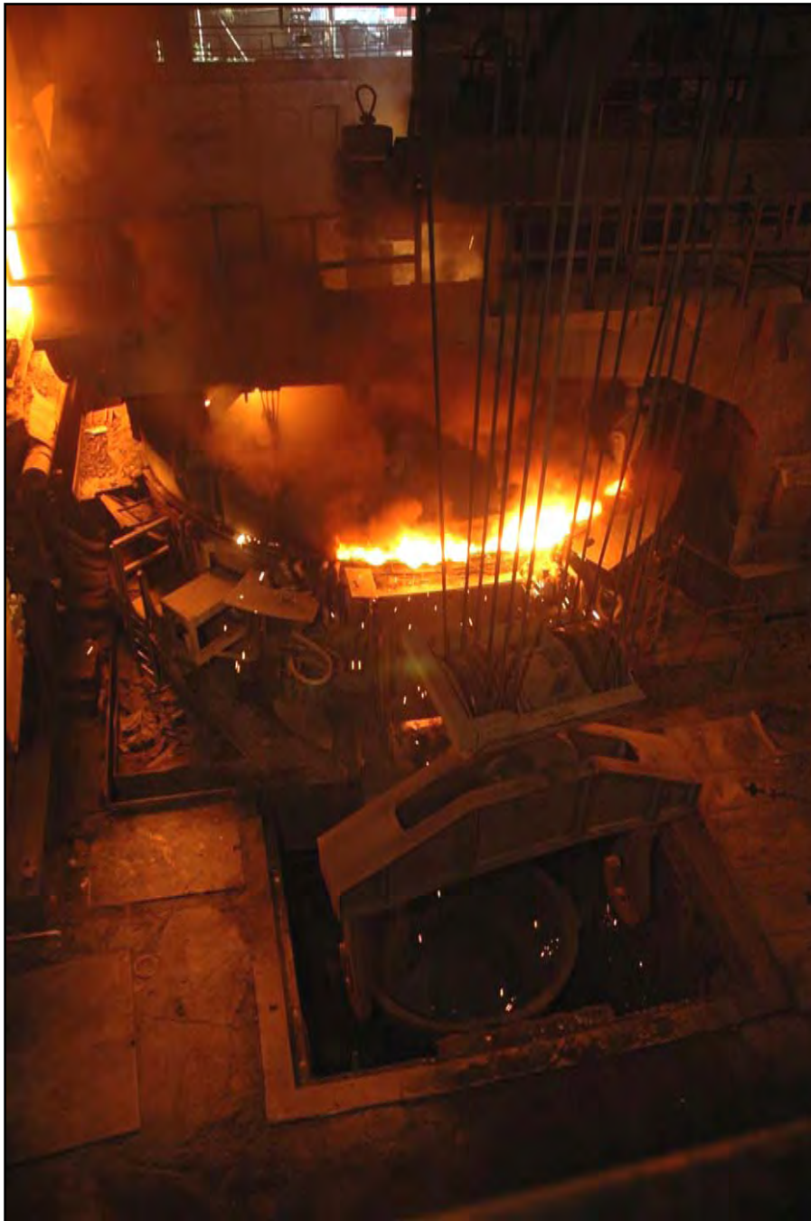
Plate 54: Prior to de-slagging a ladle is lowered into position below the slagging door
