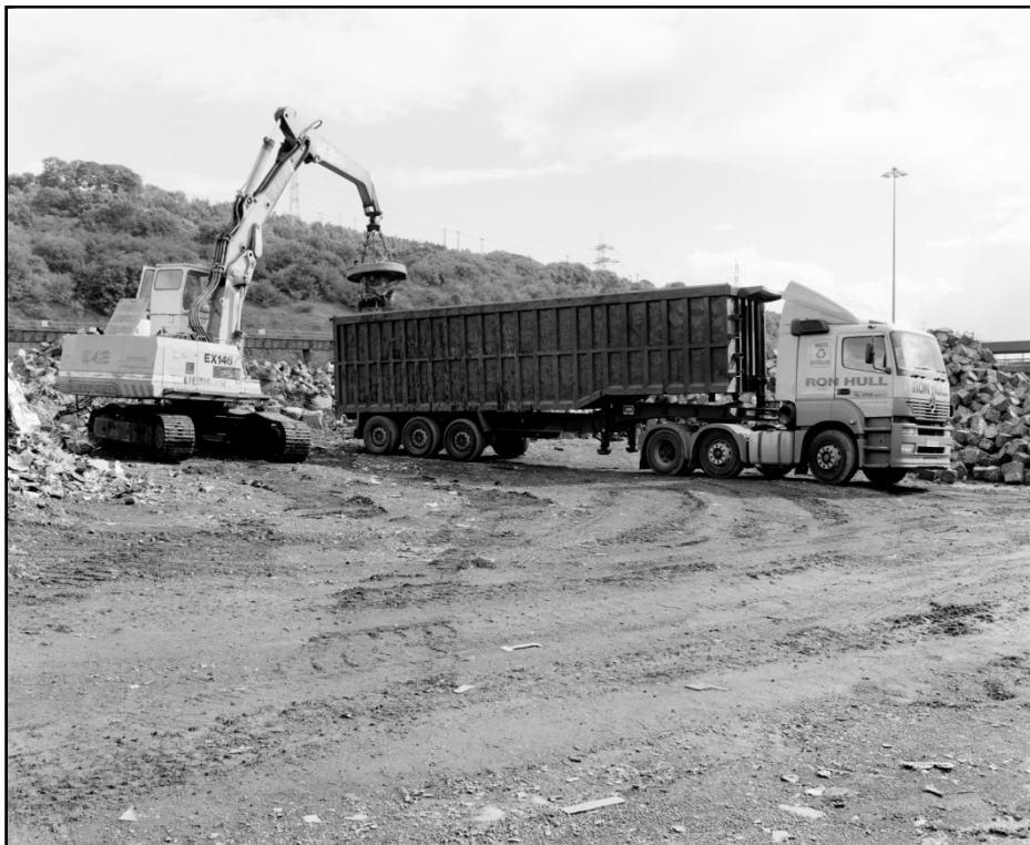
Plate 8: Details of electromagnetic loading of scrap (film 13:1)
