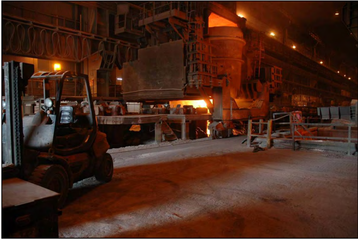
Plate 62: The molten steel is teemed into moulds
