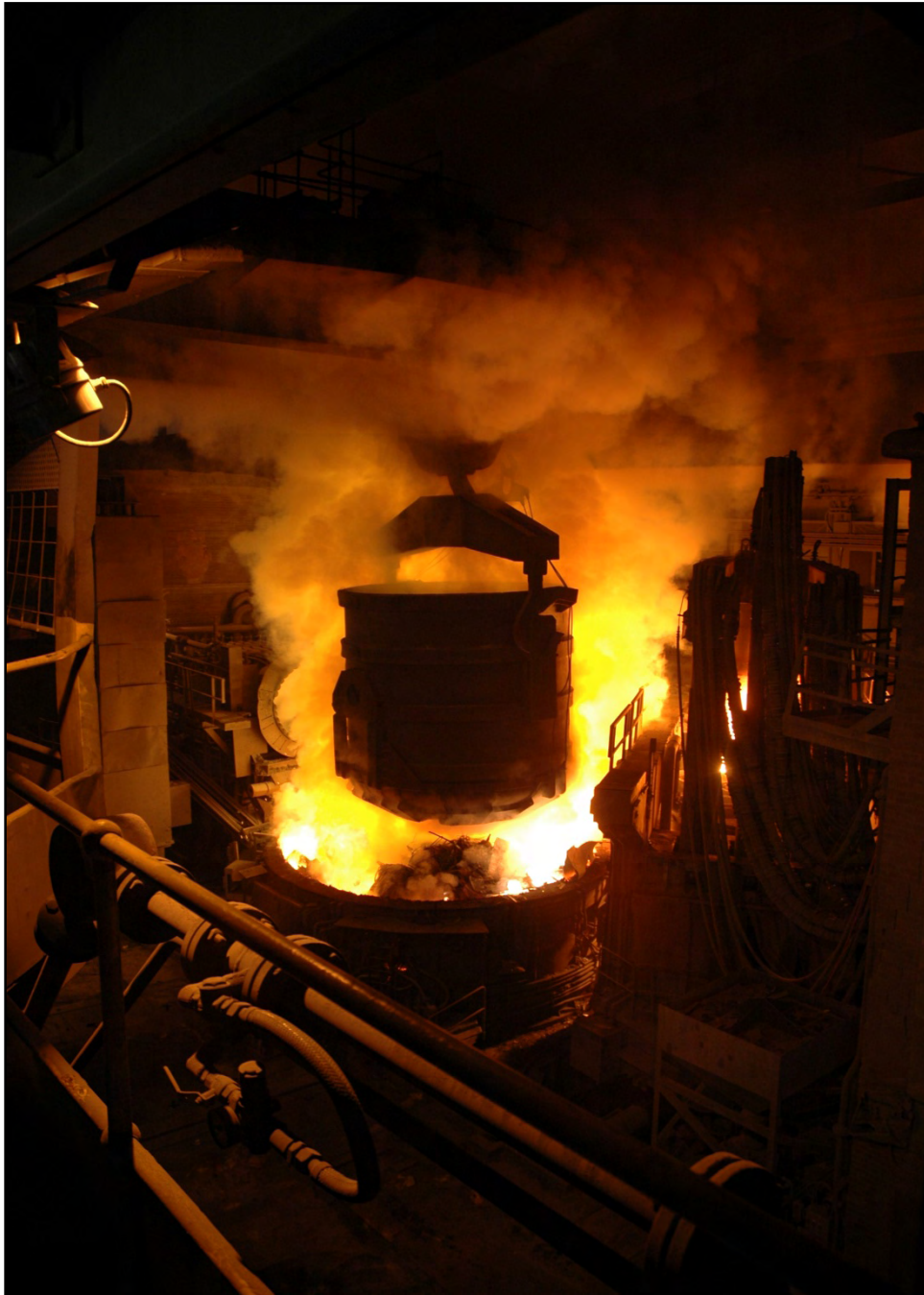
Plate 40: The clamshell doors of the basket are opened and the scrap steel is deposited into the furnace
