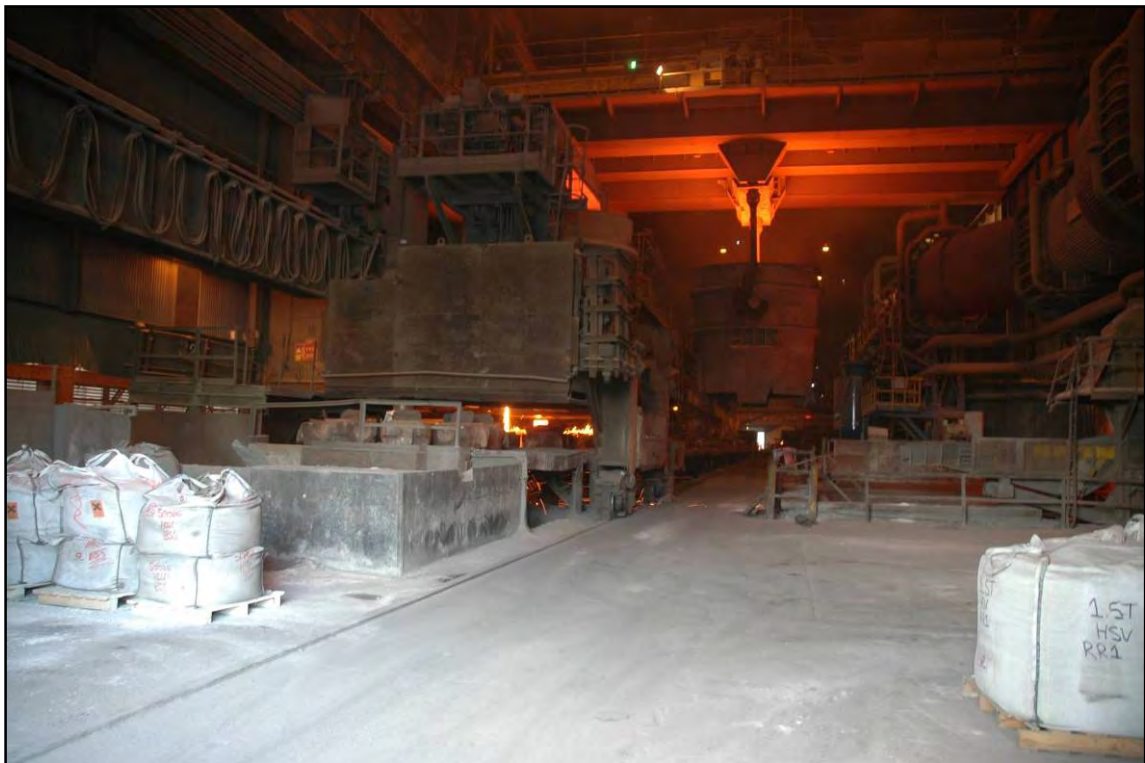
Plate 61: The ladle is transferred to the teeming area
