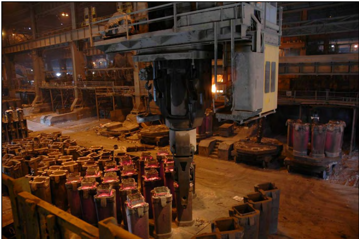
Plate 63: On cooling, an overhead crane is used to move the moulds and the stainless steel ingots are removed
