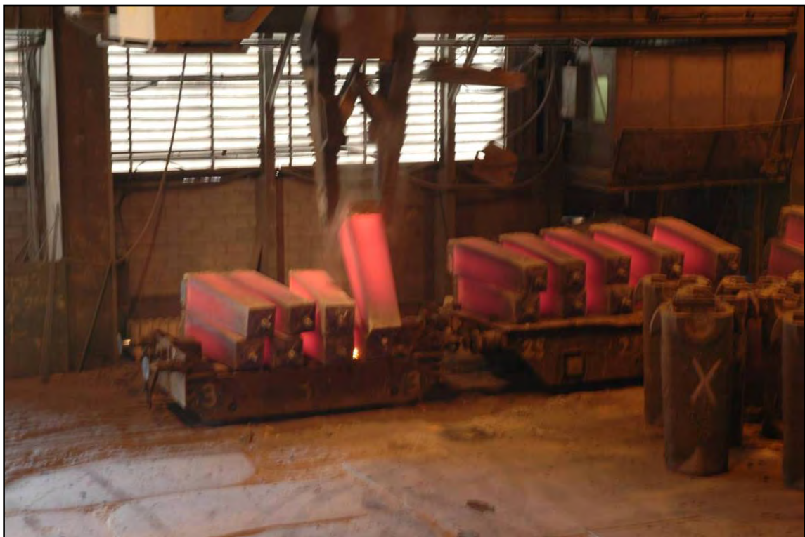
Plate 64: The finished ingots are loaded on to flat bogies for transfer from the melting shop
