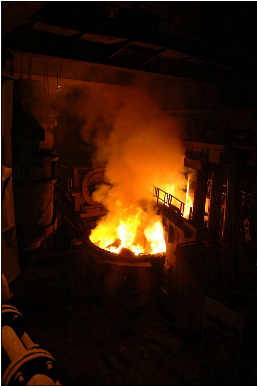
Plate 48: The second charge of scrap steel begins to glow
