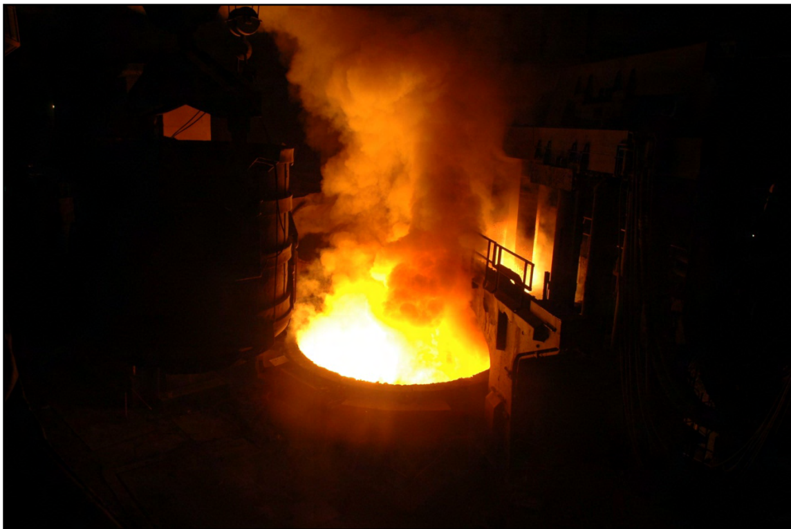
Plate 39: Detail of electric arc furnace within melting shop, showing the furnace roof being opened and a charging basket being manoeuvred into position above the furnace shell.
