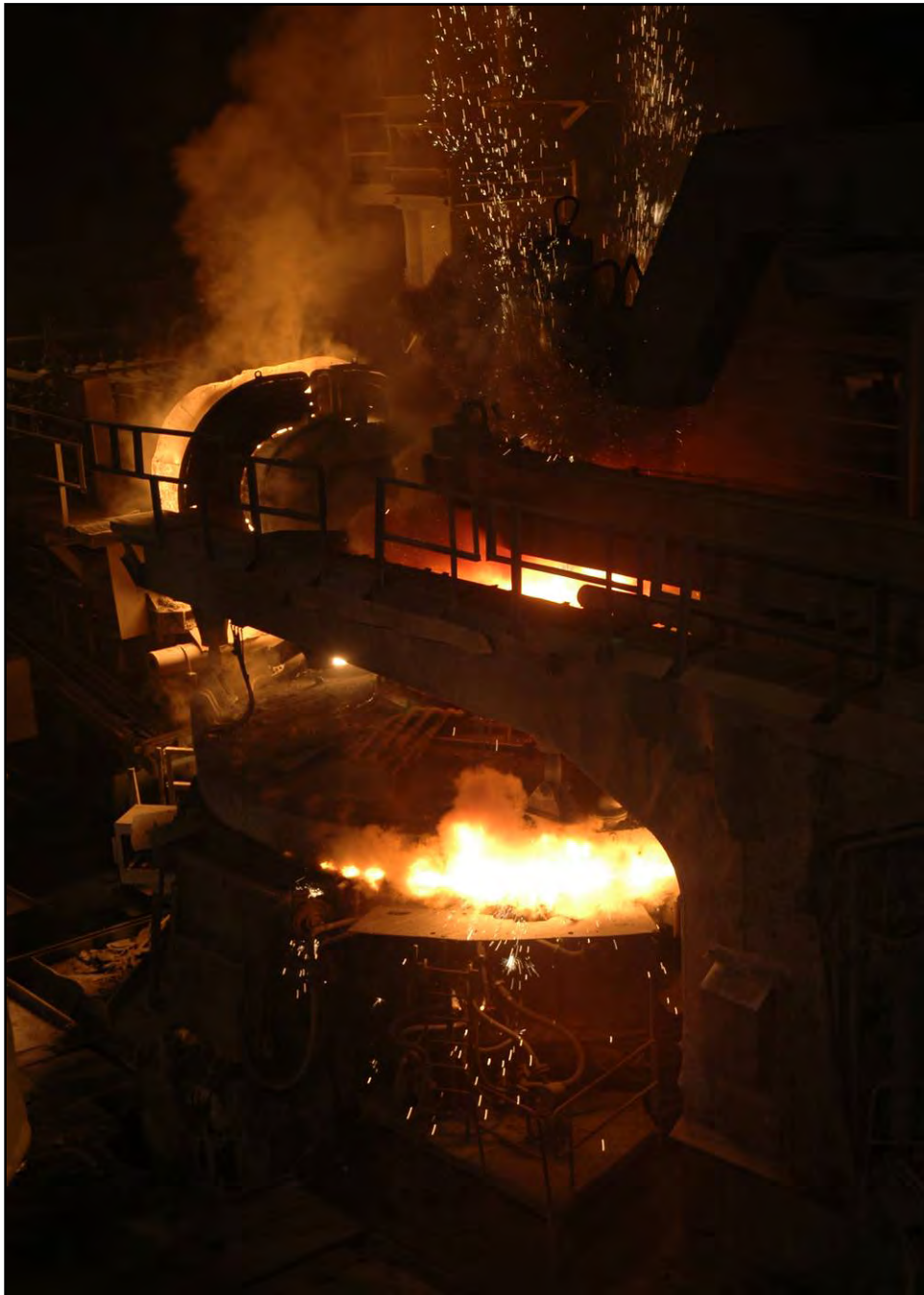
Plate 45: The electrodes are withdrawn and the roof of the furnace is opened to receive a second charge
