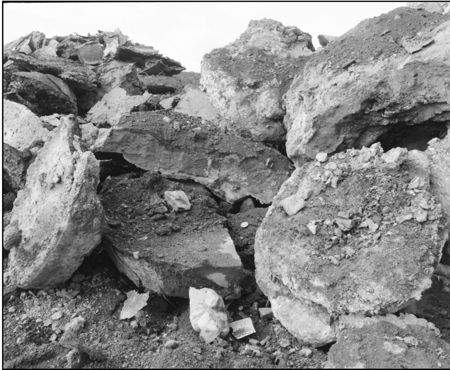
Plate 29: Scrap waste from melting knocked out from base of previous melts (film 13:4)
