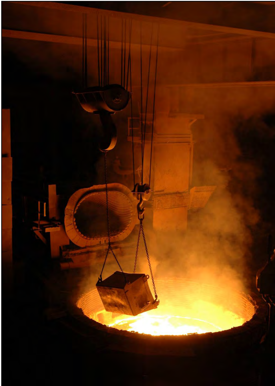
Plate 53: The limestone causes the formation of slag on the surface of the melt
