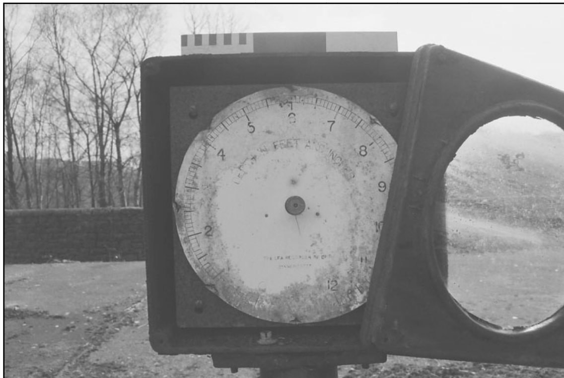
Plate 14: Detail of western depth gauge; note depth registers up to 12ft (film 1.08)
